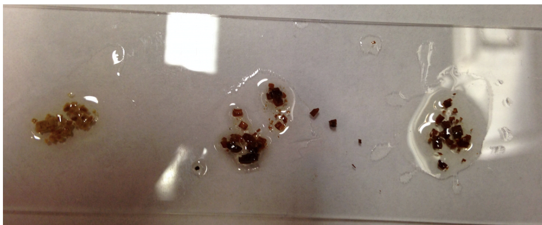
Figure 4.26. Picture of IRMOF-9-dcppy- \text{NH}_2 (left), IRMOF-9-Ir-dcppy- \text{NH}_2 (middle), and IRMOF-9-Ir-dcppy- \text{NH}_2 after 1 catalytic cycle (right), showing the color change of MOF crystals after cyclometalation reaction.
