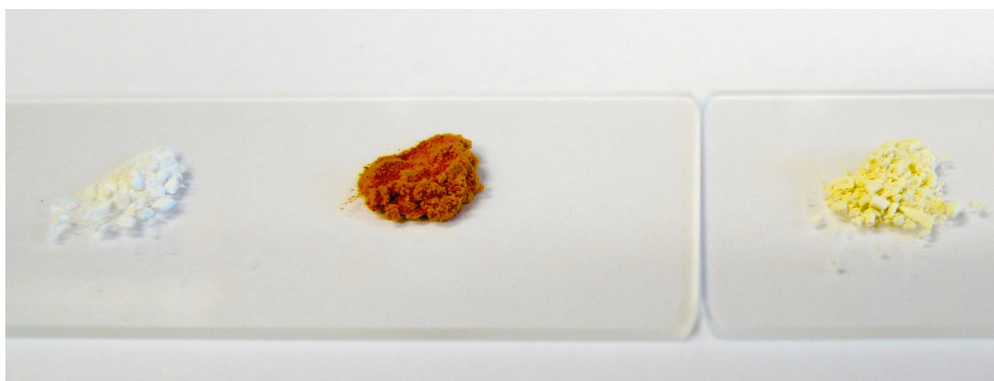
Figure 3.5. Picture of UiO-67-dcppy (left), UiO-67-Irdcppy (middle, containing 7.7 wt% of Ir), and UiO-67-Rhdcppy (left, containing 5.4 wt% of Rh).
