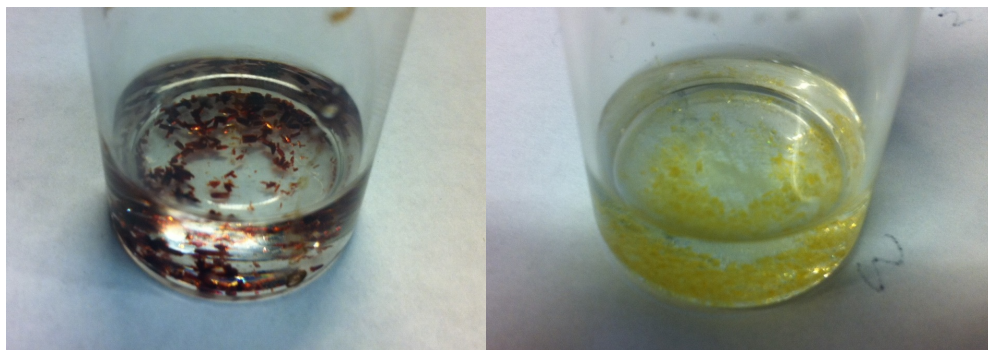
Figure 3.2. Picture of DMOF-1-Irdeppy (right, containing 8.3 wt% of Ir) and DMOF-1-Rhdeppy (left, containing 7.4 wt% of Rh).
