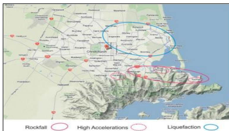
Figure 8: Approximate location of the worst types of damage during the 2011 Christchurch Earthquake (Buchanan et al. 2011)
