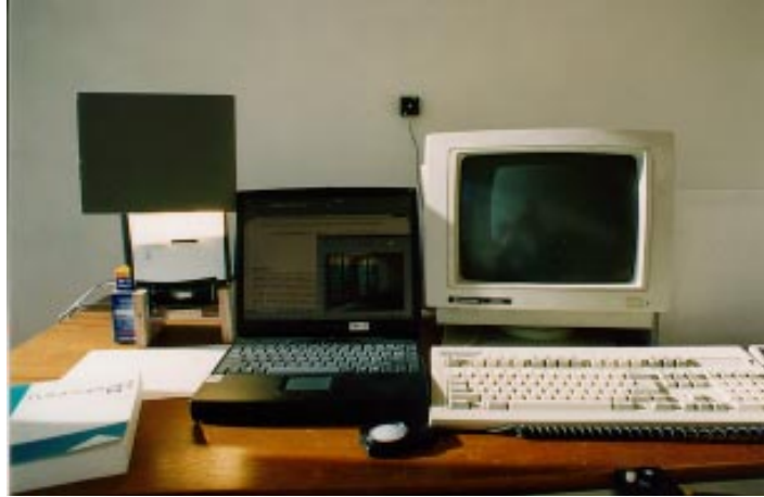
Fig. 9. Veiling reflections and direct sun on a CRT versus an LCD computer screen.
