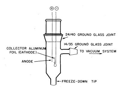
Fig. 7. Glow discharge tube used to deposit xenon on aluminum foils.
