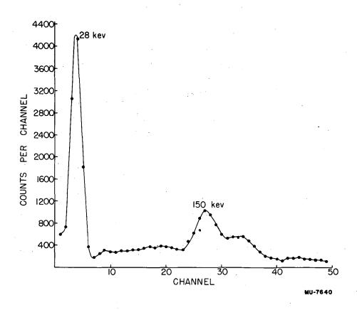
Fig. 4. Gamma spectrum of  $Xe^{123}$  sample isolated from  $Cs^{123}$ .
