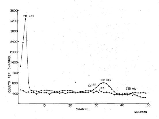
Fig. 3. Gamma spectrum of Xe<sup>122</sup>-I<sup>122</sup> mixture and on pure I<sup>122</sup> showing assignment of 180 kev gamma radiation to Xe<sup>122</sup>.
