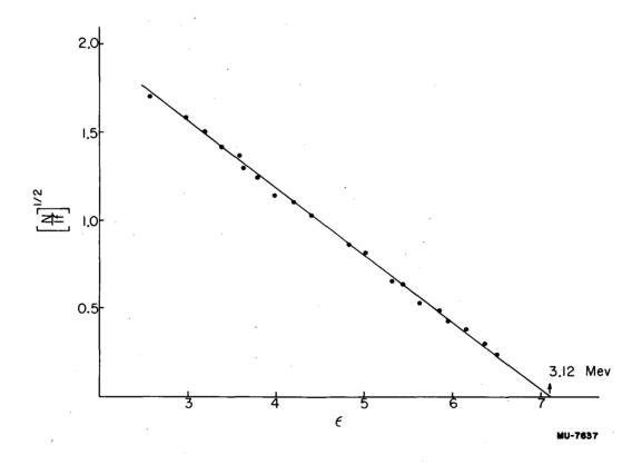
Fig. 1. Fermi-Kurie plot of positron spectrum of I<sup>122</sup> obtained on Xe<sup>122</sup>-I<sup>122</sup> sample.
