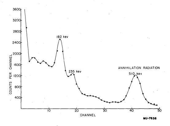
Fig. 2. Gamma spectrum of Xe<sup>122</sup> taken on scintillation spectrometer.
