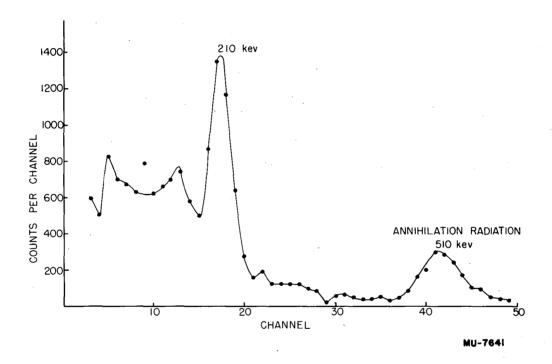
Fig. 5. Gamma spectrum of  $I^{121}$ .
