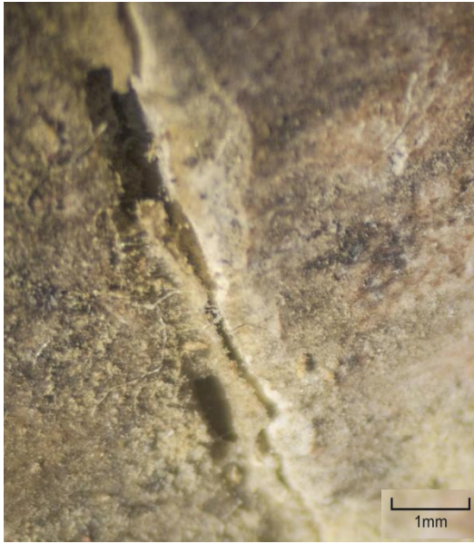
Figure 3: Delamination of ceramic material in a crack.
