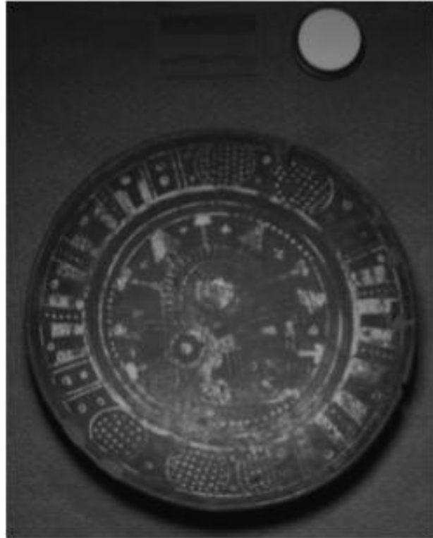
Figure 12: Ultraviolet ( \lambda_{exc} \text{ max} = 365 \text{ nm} ) Reflectance ( \lambda 300 - 400 \text{ nm} ) of the bowl's decoration before treatment. Captured with a modified Nikon D90 DSLR camera with a Peca 900 filter.
