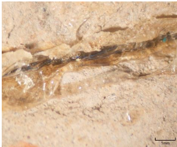
Figure 4: Photomicrographs showing that there is excess adhesive along the joins and that the adhesive is shrinking and pulling apart the ceramic fabric at the joins.
