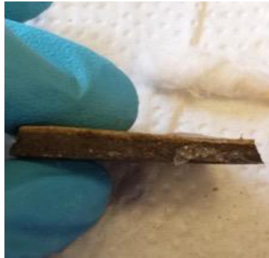
Figure 6: Once softened, the adhesive could be picked and peeled off of the break edges.
