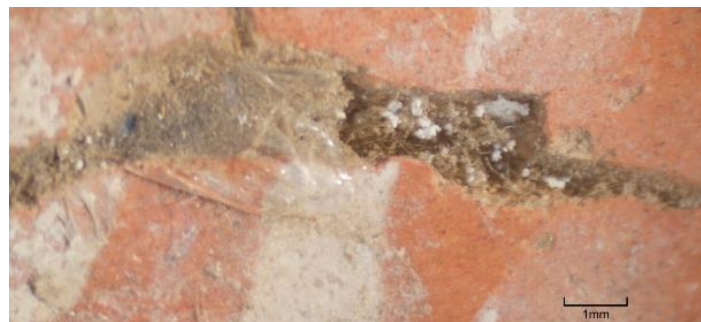
Figure 8: Photomicrograph showing a join with excess adhesive, dust/dirt, and white particulate.
