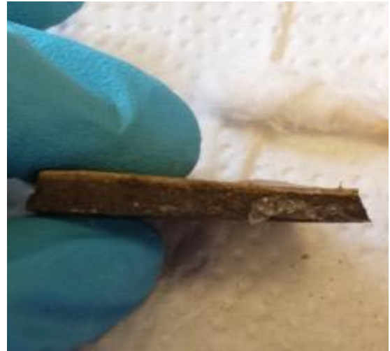
Figure 5: Once softened, the adhesive could be picked and peeled off of the break edges.
