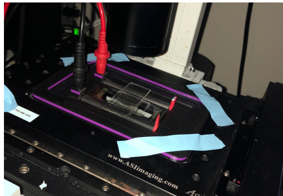
Figure 2-2. Orthogonal view of the ultrathin IEF assay assembly on a widefield epifluorescence microscope.
