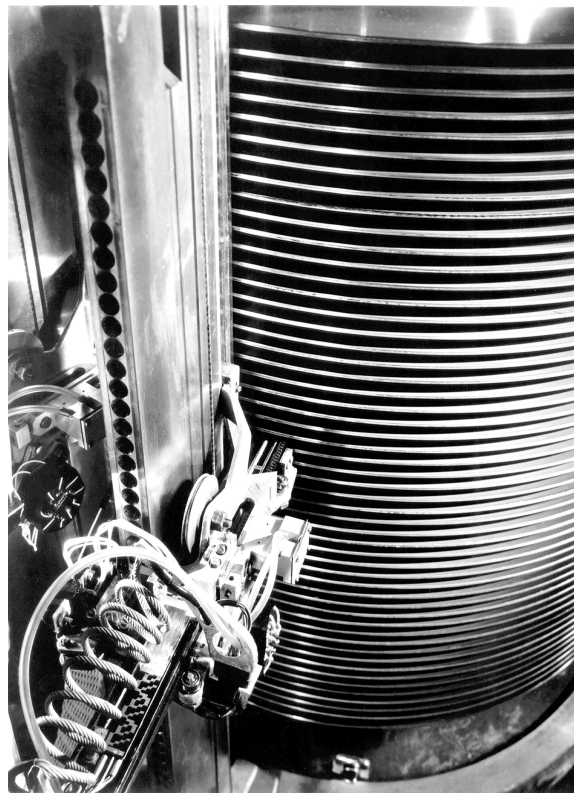
Figure 1.1 The IBM 350 Disk Drive (with permission from Hitachi Global Storage Technologies).
