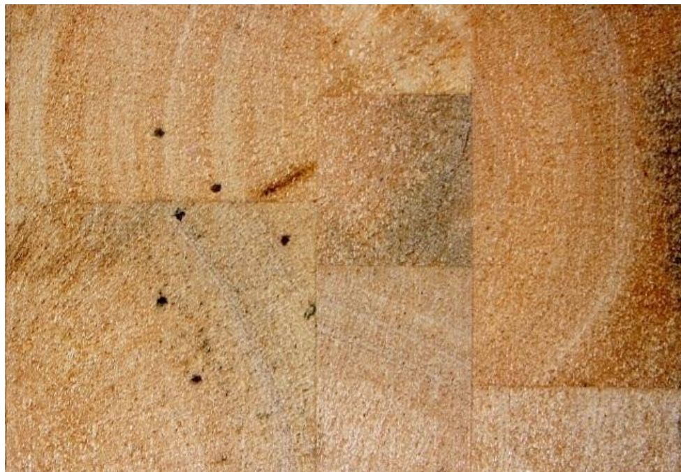
Figure 46. Non-homogeneity of balsa wood core
