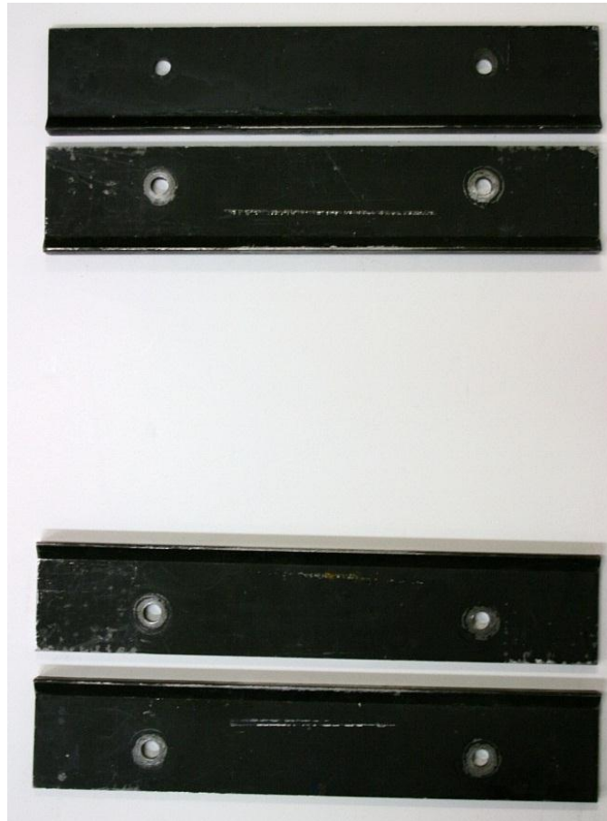
Figure 90. V-clamps provide simply supported boundary conditions
