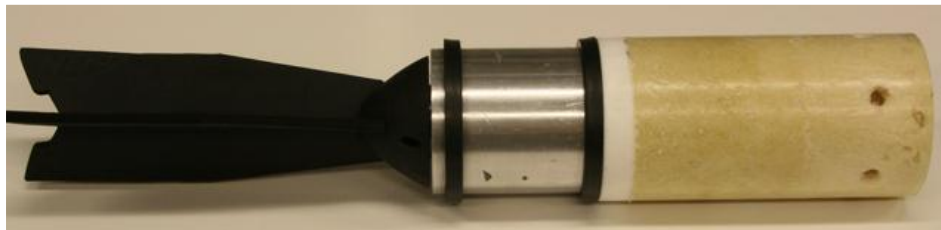
Figure 71. Fully constructed PPGP
