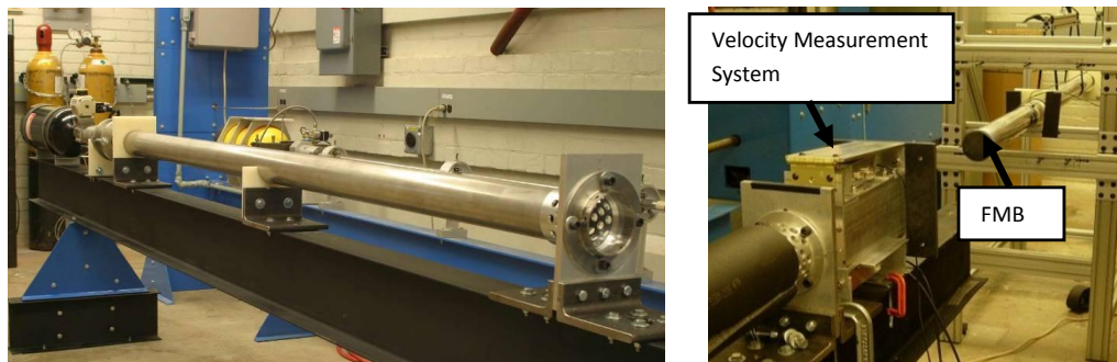
Figure 17. Gas gun and force measurement bar setup
