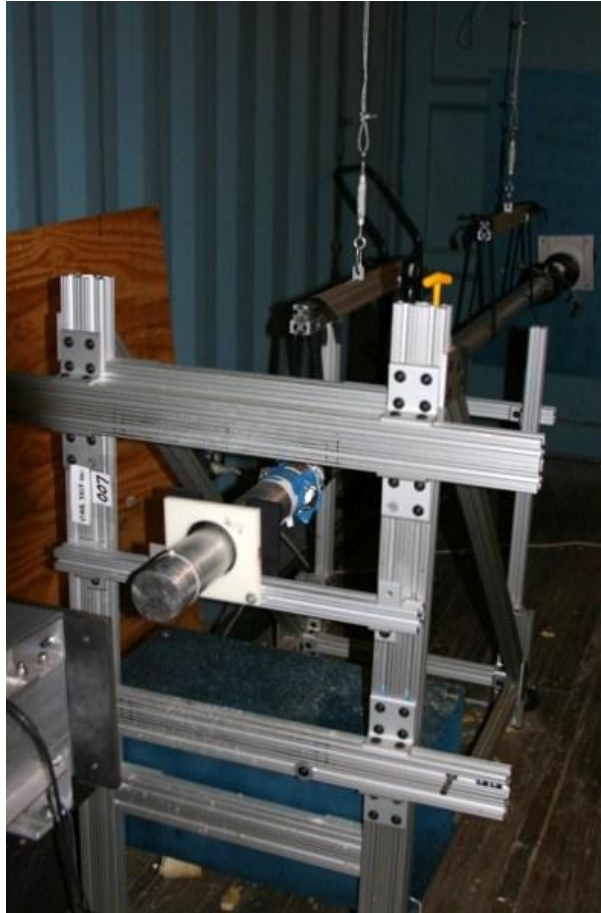
Figure 82. Hopkinson bar (FMB) and aluminum test fixture frame
