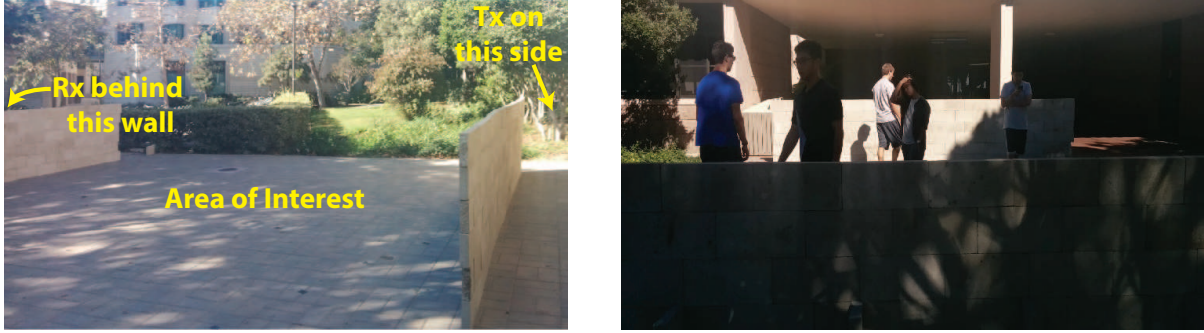
Figure 3.18: (left) The second area of interest between two concrete walls (Area 2), and (right) an example where people are walking in between these walls. The WiFi nodes are located outside of the area of interest, behind the walls, as indicated in the left figure. Readers are referred to the color pdf for better visibility.
