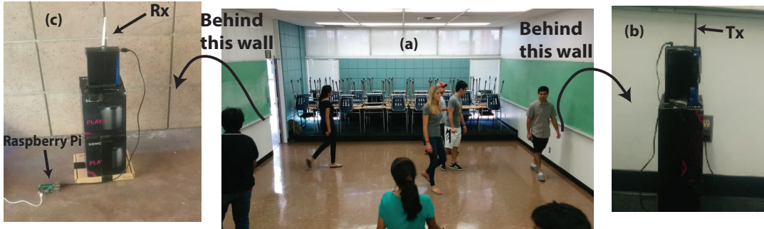
Figure 3.16: (a) The first area of interest (Area 1), a closed classroom on our campus with wall made of concrete, where people are walking, (b) the Tx WiFi node located outside the classroom, behind one of the walls of the classroom as marked, and (c) the Rx WiFi node, along with the Raspberry Pi board that is used to control the data collection, which is located outside of the classroom behind the wall that is indicated.
