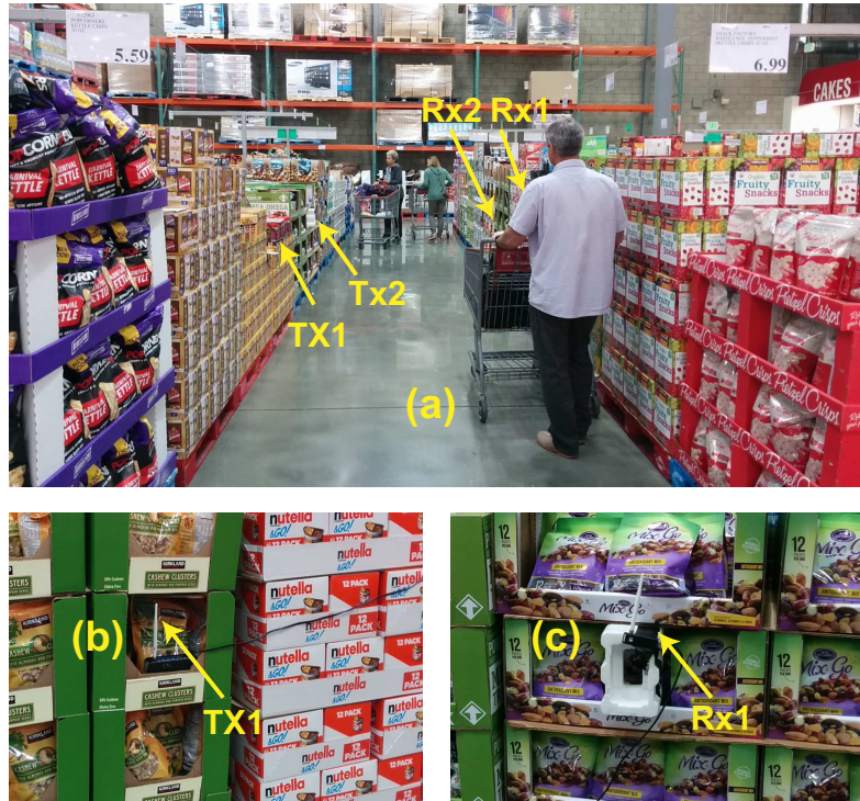
Figure 4.15: The Costco experiment – the figure shows the considered “snacks and cookies” aisle in Costco along with a pair of WiFi links positioned along the aisle to make wireless measurements.
