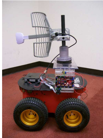
Figure 2.1: The figure shows a Pioneer 3-AT robot with the additionally-mounted servomechanism and a directional antenna.
