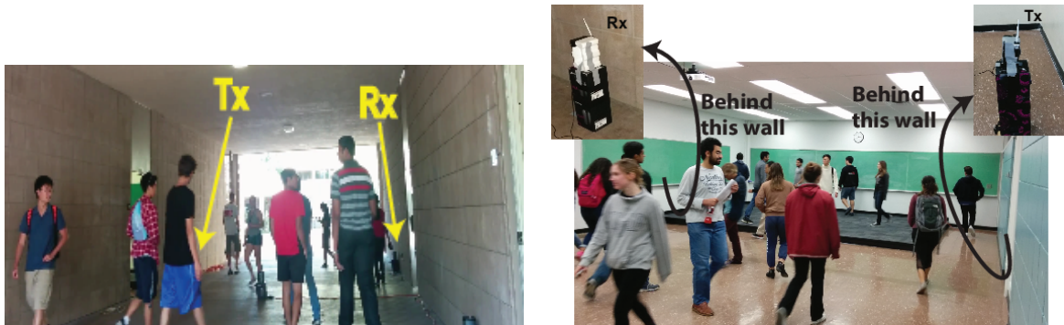
Figure 1.2: A stationary WiFi transmitter and receiver are tasked with determining the number of people in the area based on only the received power measurements over a short period of time. (left) Considers a scenario where the Tx and Rx are located in the same area where people are walking, while (right) considers a scenario where the Tx and Rx are located outside a building while people are walking inside.
