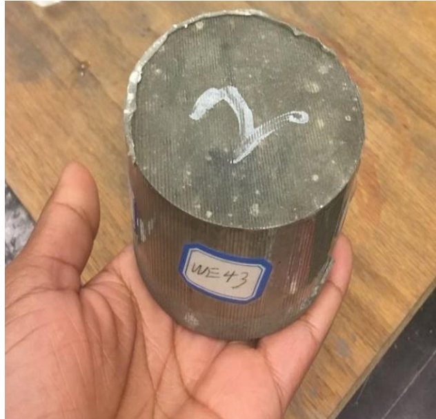
Figure 2.1 Piece of WE43 magnesium alloy produced by melting and casting process.
