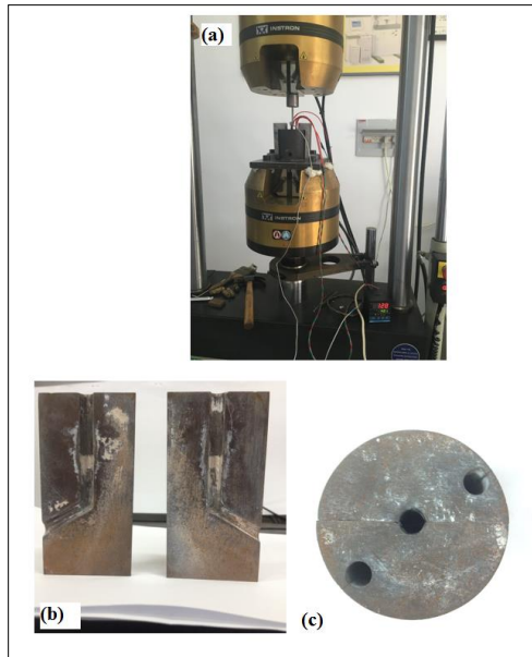
Figure 2.5 (a) ECAP system (b) transversal view of the die (c) view from the top of the die
