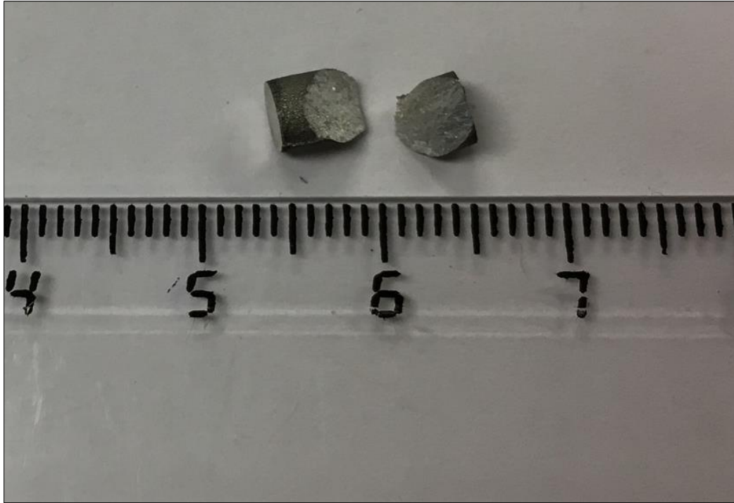
Figure E.7 Fracture surface of quasi static compression test \Sigma\varepsilon = 2.15 on y-axis
