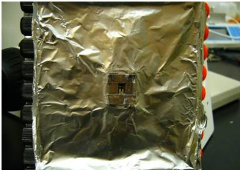
Figure 4.17: Microfluidic chip shown embedded within the faraday cage. Optical window was included to allow microscopy.
