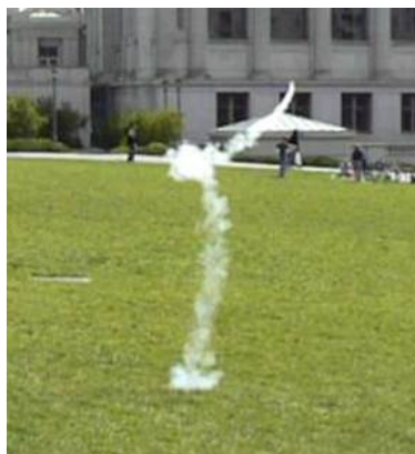
Figure 3.1: In the absence of aerodynamic forces, a bare solid rocket engine spins out of control. A stabilizing controller is therefore necessary on a minirocket LV.
