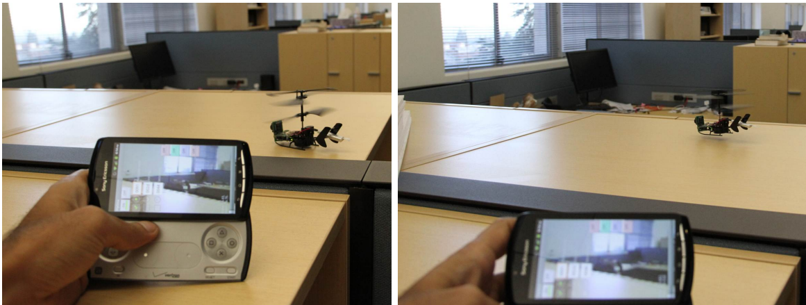
Figure 5.3: An experimental realization of figure 5.1 above passes downstream communication and upstream sensor data along a multi-modal multi-hop network path consisting of 3G, wifi, and 802.15.4 links.
