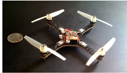
Figure 2.18: The mini quadrotor developed by Daedalus Flight Systems and UMD uses the GINA hardware, but modifies the firmware to include an on-board attitude stability loop to control its four brushless DC motors.
