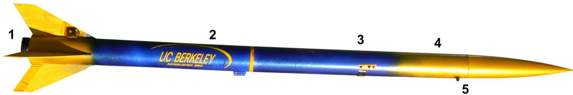
Figure 3.7: An updated rocket designed and built by Florian Kehl contained a GINA mote for full 6 axis inertial sensing, along with 3 axis attitude control with 4 channel flywheel and gimbaled nozzle actuation.
