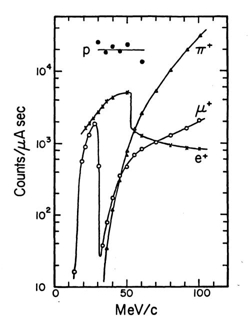
FIG. III.3. Positive particle fluxes versus beamline momentum settings in the M13 beamline at TRIUMF (taken from Ref. 26). The data was collected with all slits and jaws in the beamline fully open.
