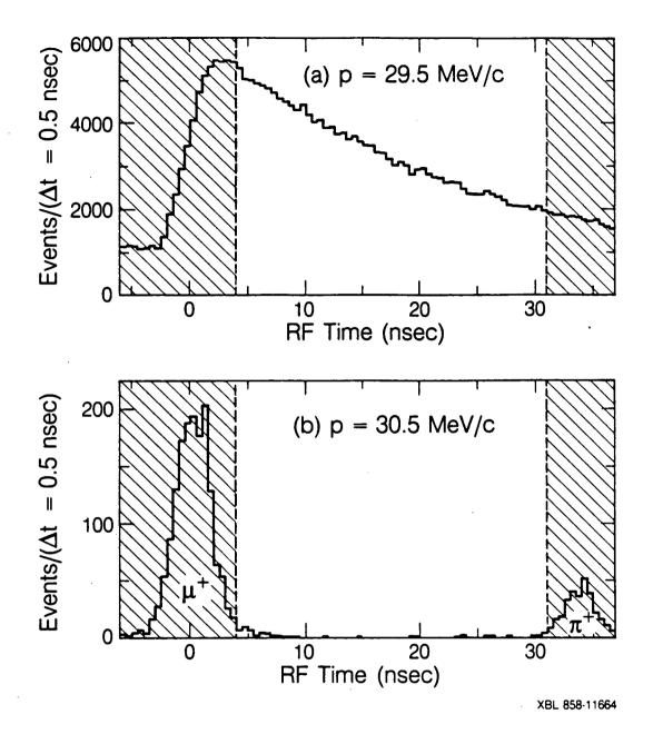
FIG. III.4. Beam particle arrival times at the stopping target with respect to the cyclotron RF cycle at (a) 29.5 MeV/c and (b) 30.5 MeV/c. The shaded regions, containing almost all of the cloud  $\mu^+$  and prompt  $\pi^+$  contaminations, were rejected.
