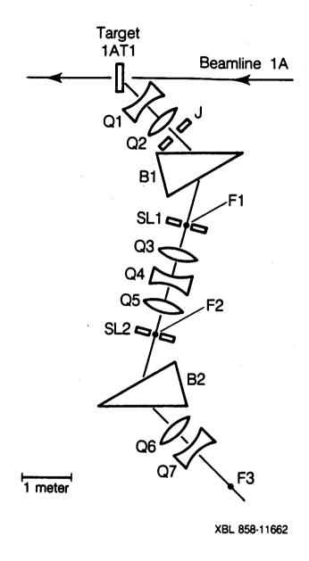
FIG. III.2. The M13 beamline at TRIUMF. B1 and B2 are dipoles; Q1-Q7 are quadrapoles; F1-F3 are foci; the slits SL1 and SL2, and the jaws J have both horizontal and vertical components.
