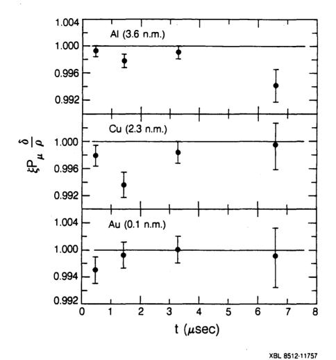
FIG. V.4. The results for  $\xi P_{\mu} \delta/\rho$  evaluated in four muon decay time ranges for the three metal targets, Al, Cu and Au, constituting 93% of the data. Only statistical errors are shown. The results are plotted versus t, given by equation (5.12). The target material
