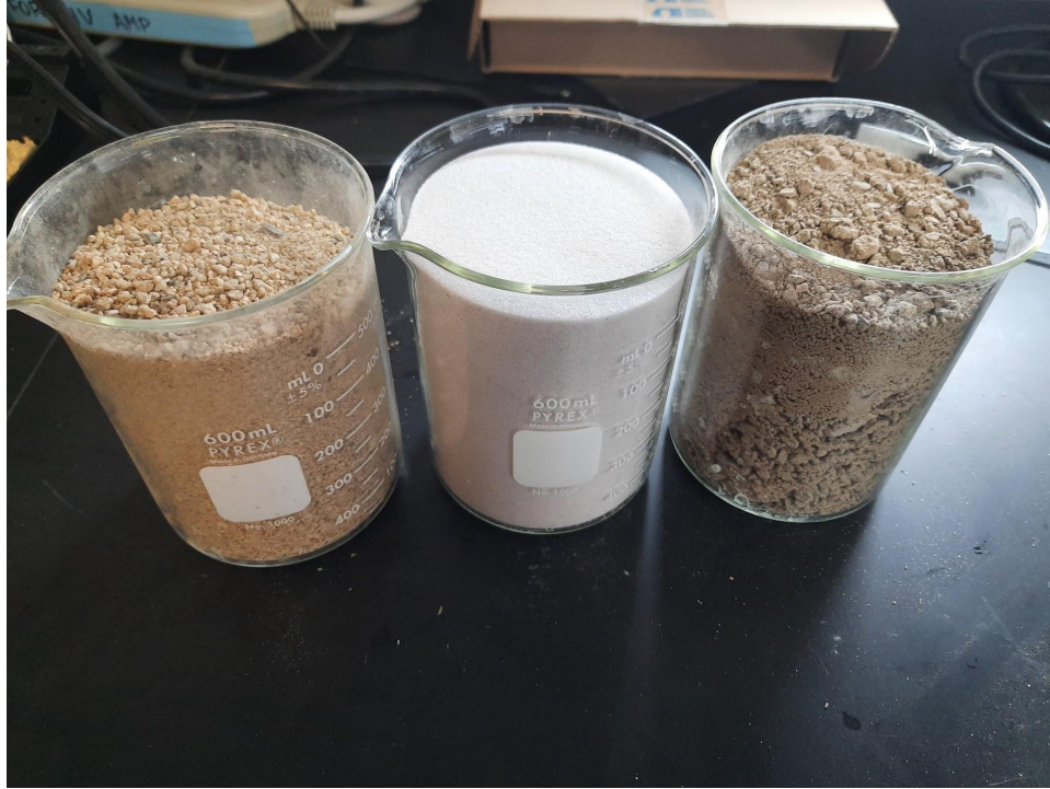
Figure 11. The figure displays the different sediments used in the study to validate the performance of the H-beam structure for different sediment types. The sediments include regular sand, Ottawa F-65 silica sand, and regular soil
