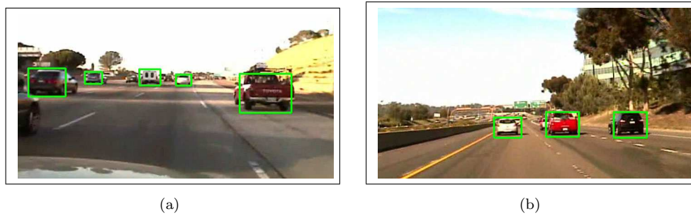
Figure 3.11: a) Recognition output in shadows. Five vehicles were detected, and two were missed due to their distance and poor illumination. We note that poor illumination seems to limit the range of the detection system; vehicles farther from the ego vehicle are missed. b) Vehicle recognition output in sunny highway conditions.
