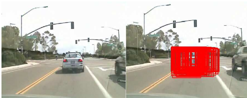
Figure 3.12: Left: The vehicle in front was not detected in this frame on a cloudy day, due to smudges and dirt on the windshield. Right: The vehicle's track was still maintained in the following frame.
