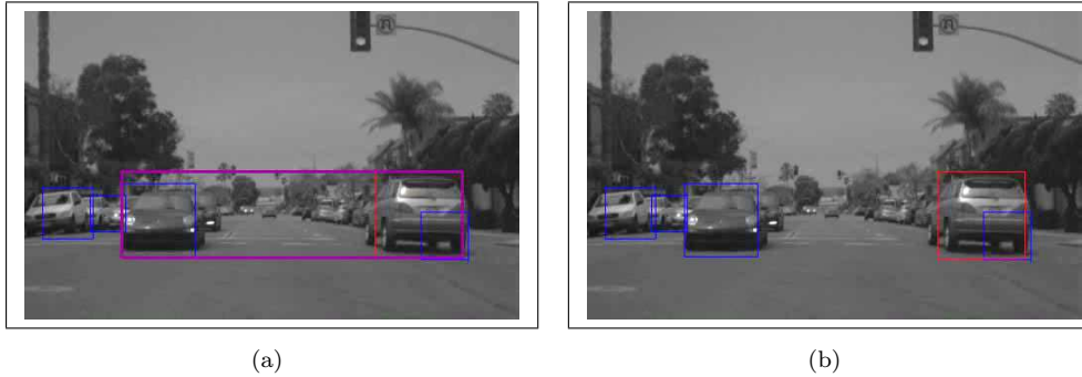
Figure 6.6: Using the tracking velocities of the vehicle parts eliminates erroneous side-view vehicles. a) A side-view vehicle is erroneously constructed from an oncoming and a preceding vehicle. b) Using velocity information from tracking, the erroneous side-view vehicle is not constructed.
