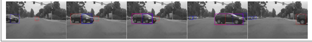
Figure 6.7: Showing the full track of a vehicle in the camera’s field of view. In the first frame, the front part of the vehicle is detected, but most of the vehicle is occluded. A couple of frames later, the rear part of the vehicle is detected as well. The full side-view vehicle is detected, and identified with a purple bounding box. The vehicle and its parts are tracked while they remain in the camera’s field of view. As the vehicle leaves the camera’s field of view, its rear part is still detected.
