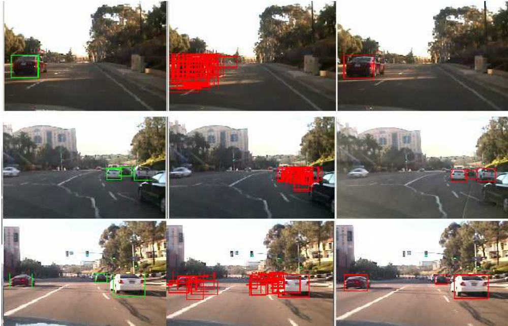
Figure 3.7: Left: Detector outputs for a single vehicle [top], and multiple vehicles [middle and bottom]. Middle: Multiple location hypotheses generated by the Condensation filter. Note the multi modal distribution of the hypotheses when tracking multiple vehicles [bottom]. Right: Best tracking results, as confirmed by detections in the consequent frame.
