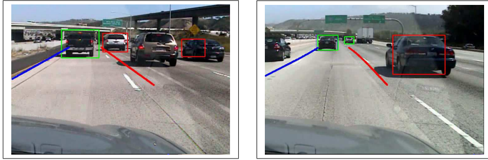
Figure 5.10: a) Poor lane localization due to a missed vehicle detection. The missed vehicle detection leads the lane tracker to integrate erroneous lane markings into the measurements, resulting in worse lane estimation for the right marker. b) Example misclassification of lane position. The jeep in the right lane [green] has been classified as in the ego lane. This is due to the fact that the jeep is farther ahead than the lane tracker’s look-ahead distance.
