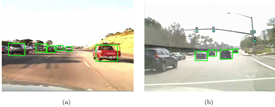
Figure 3.15: a) Recognition output in a non-uniformly illuminated scene. Six vehicles were detected. No false positives, and no missed detections. b) Recognition output in cloudy conditions. Note the reflections, glare, and smudges on the windshield.
