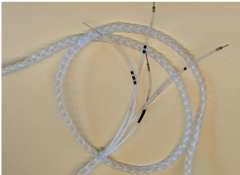
Figure C-7. Photo of Tygon microbore tubing with coding scheme in a 4-strand braid.
