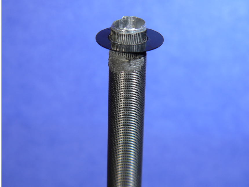
Figure 4 – The sample after the second layer of W wire was applied.
