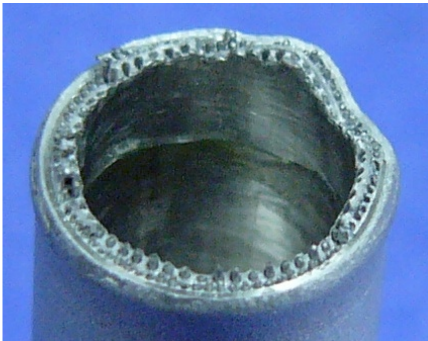
Figure 82 – Fracture surface due to tensile testing of Sample 6, Configuration 1. Notice the cone shape of the broken W rods, suggesting the W fibers supported the axial load until they fracture themselves, translating a load to the aluminum matrix.
