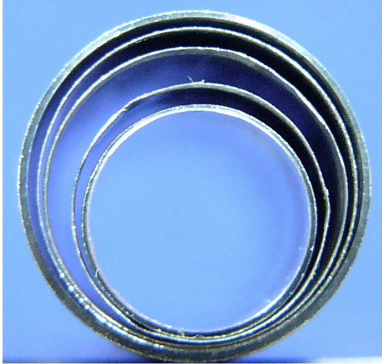
Figure 30 - Aluminum alloy 6061 tubes used to assemble Sample 1, Configuration 2. The inner and outer diameters of the tubes from the smallest to largest are: 7.5 mm and 8.1 mm, 8.6 mm and 8.88 mm, 10.08 mm and 10.36 mm, 10.84 and 11.12 mm, and 11.6 and 12.2 mm.
