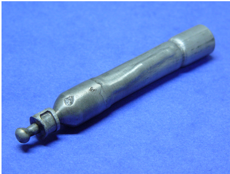
Figure 33 - Sample 1, Configuration 2 after the HIP process. Notice the bump along the entire length of the sample.
