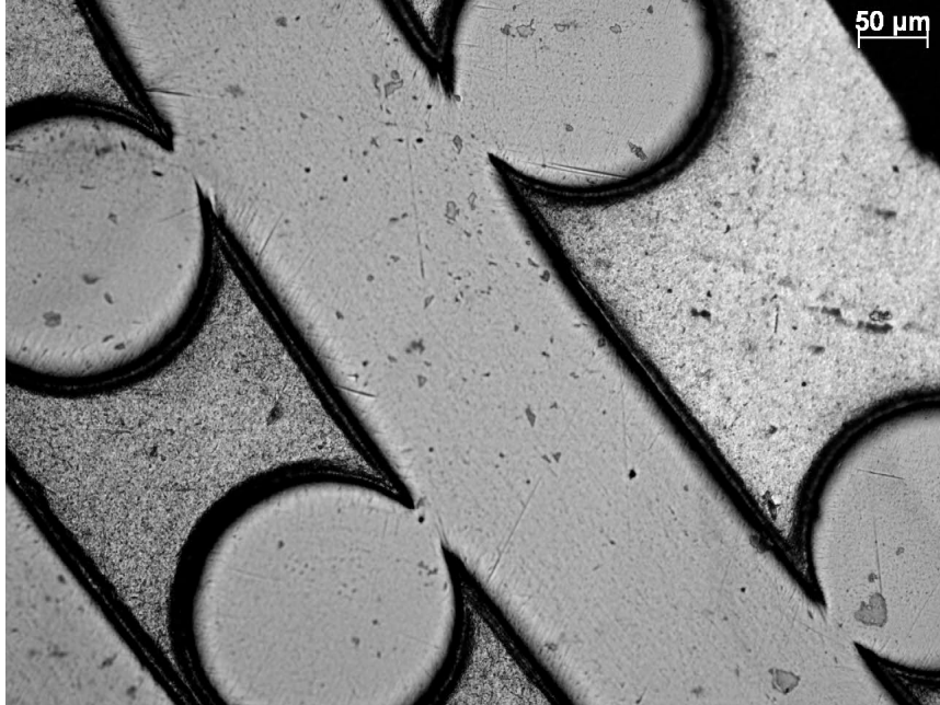
Figure 45 - Sample 4, Configuration 1 with a thicker inner tube, an optical image. Notice the contact welding between the W wire and rods.
