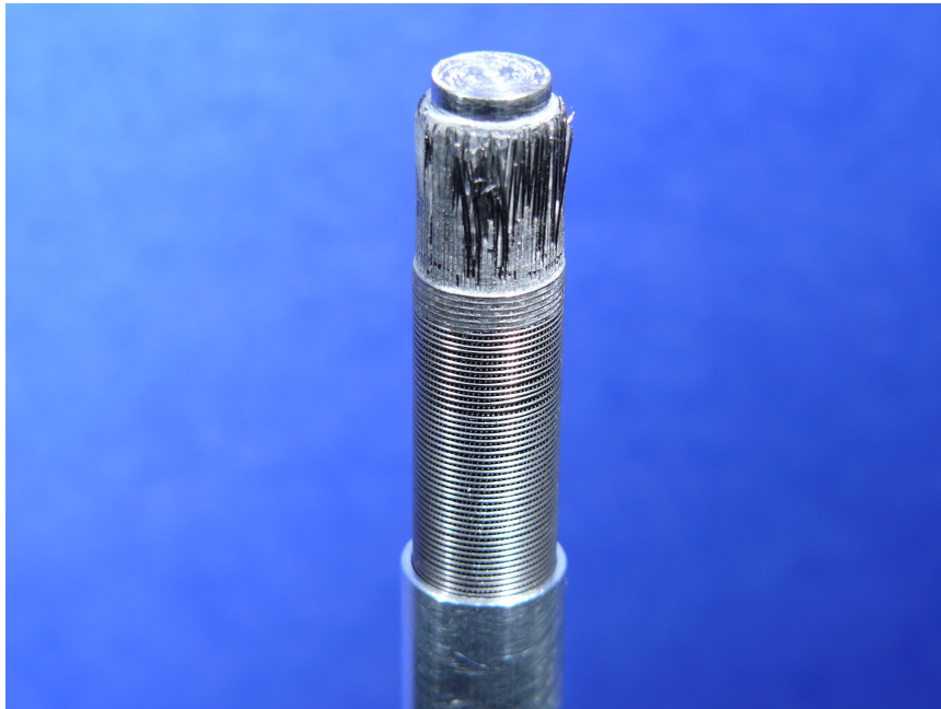
Figure 8 – Third layer of W rods applied. Notice remaining glue to keep rods and wire in place and Al guide disk. This layer was removed and redone with the forth layer of W wire.
