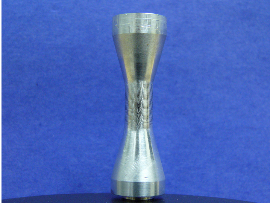
Figure 78 - Sample 5, Configuration 1 prepared for tensile testing. Notice transverse buckling in the outermost exposed W wire layer.
