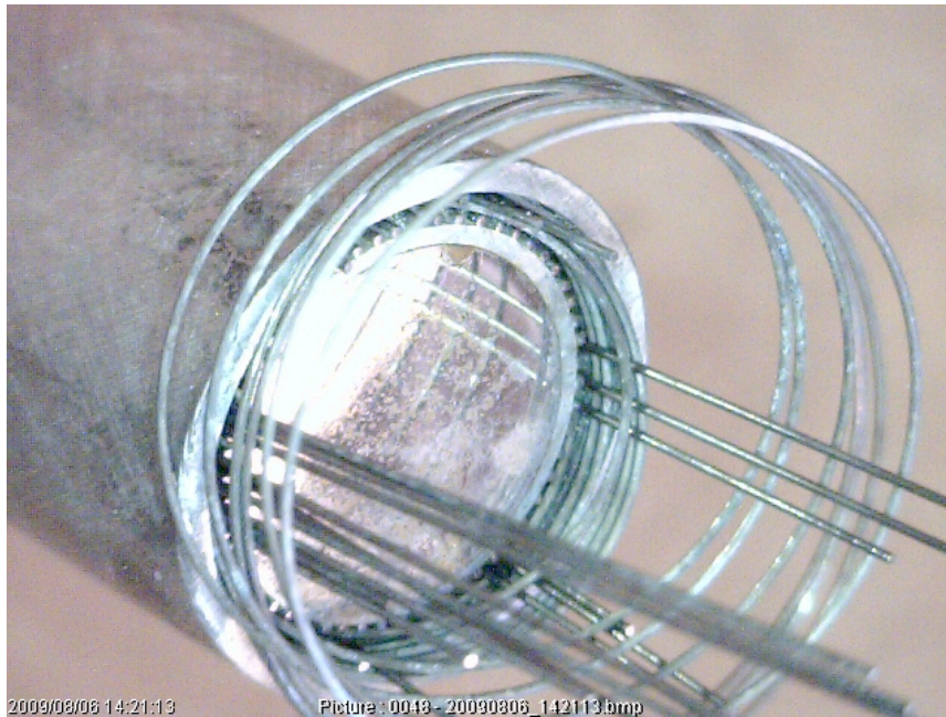
Figure 24 - Failed piece of Sample 2, Configuration 1 after 40 kHz sonication in acetone for 20 minutes.
