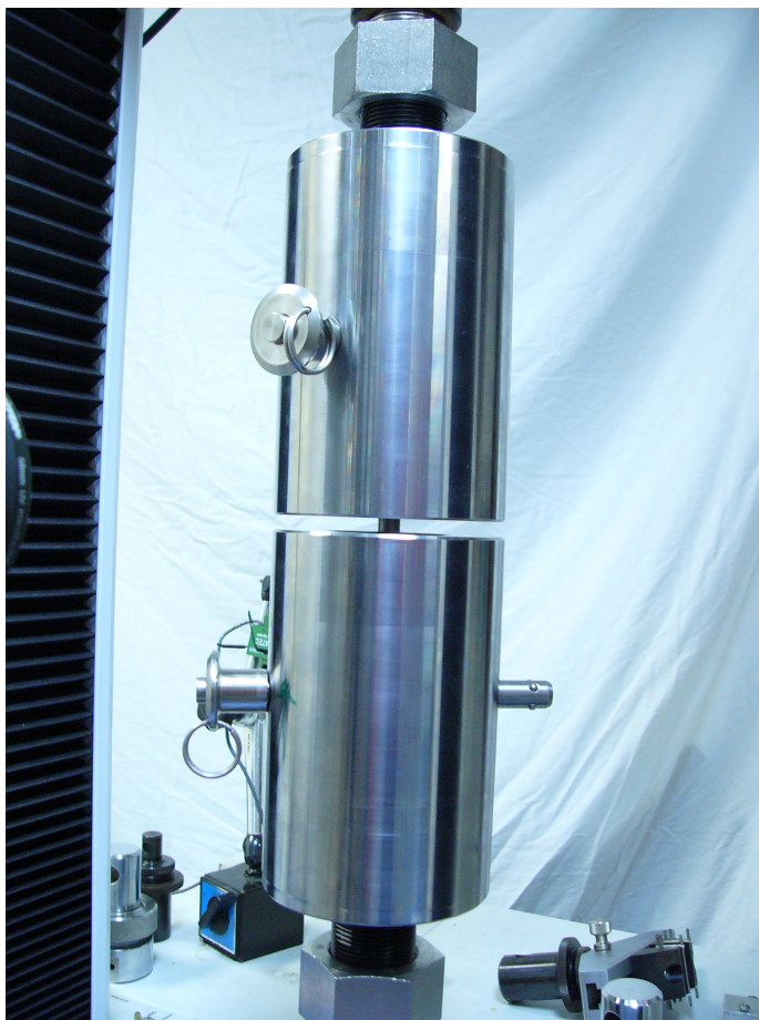
Figure 81 - Tensile test set up with steel clamps and casing holding Sample 6, Configuration 1.
