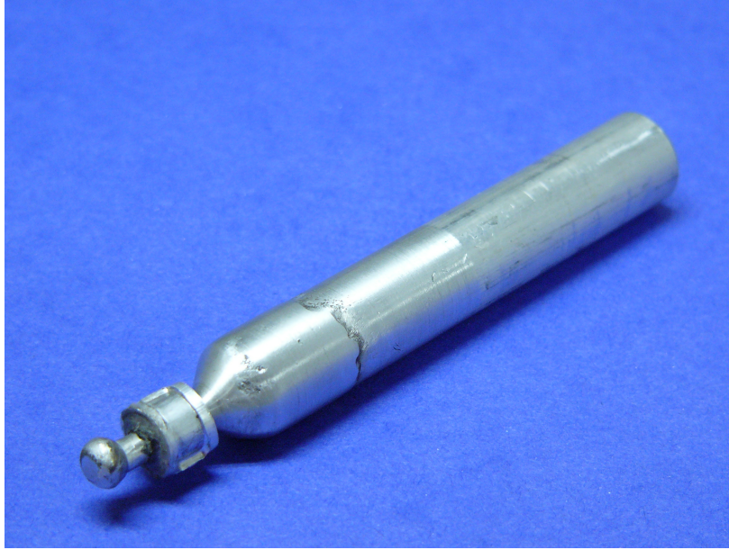
Figure 32 - Sample 1, Configuration 2 prepared within an Al 6061-T6 vacuum-sealed jacket for a HIP process.
