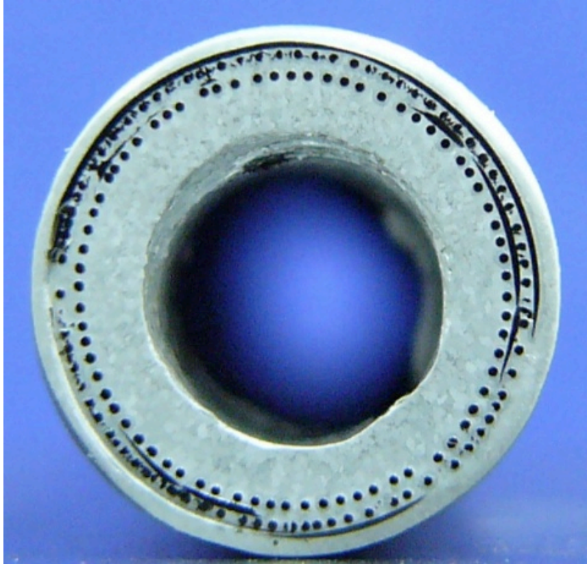
Figure 77 - Cross section of Sample 8, Configuration 4. Notice the fractured W wires to the left, causing the entire W structure to expand outward.
