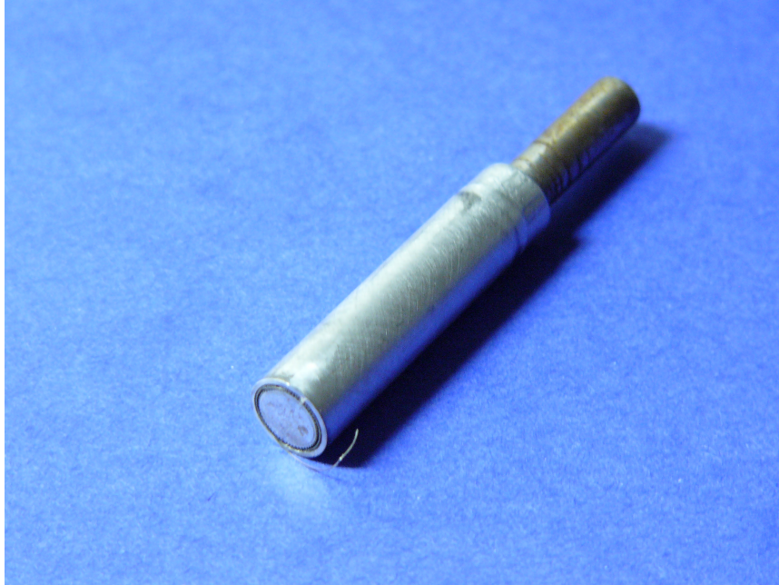
Figure 25 - Piece of Sample 2, Configuration 1 to be HIP treated after sonication in acetone for 20 minutes at 40 kHz.
