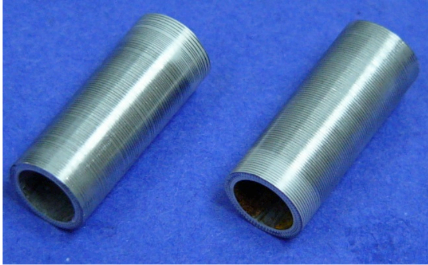
Figure 70 - Two pieces each 25 mm in length of Sample 7. Notice the irregular spacing of the exposed W wire.
