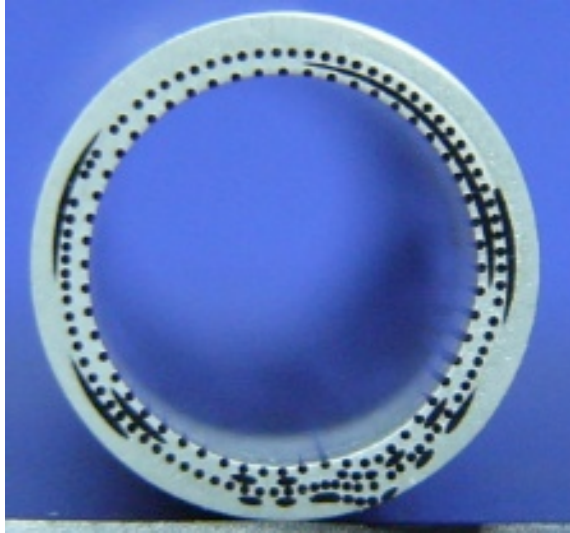
Figure 39 - Overall cross-section of Sample 4, Configuration 1 with a thicker inner tube. Notice buckled region at the bottom of the sample.
