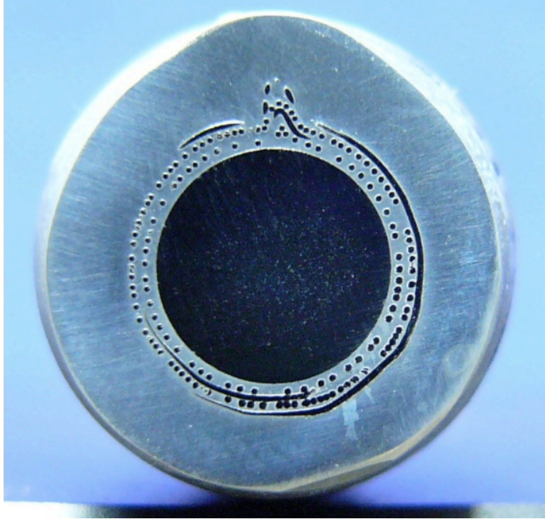
Figure 34 - Cross section of Sample 1, Configuration 1 after the HIP process. Notice the irregular W rod spacing and extreme W structure deformation at the top of the sample.
