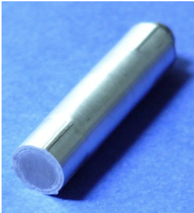
Figure 30 - Aluminum alloy 6061 tubes used to assemble Sample 1, Configuration 2. The inner and outer diameters of the tubes from the smallest to largest are: 7.5 mm and 8.1 mm, 8.6 mm and 8.88 mm, 10.08 mm and 10.36 mm, 10.84 and 11.12 mm, and 11.6 and 12.2 mm.
