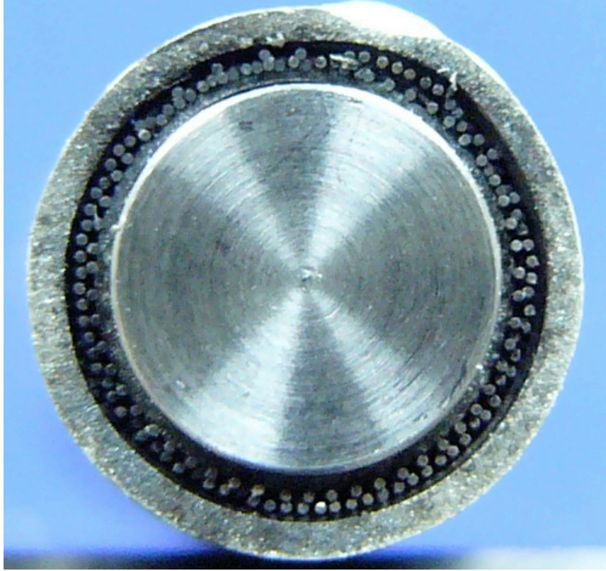
Figure 17 – Sample 1, Configuration 1 after annealing and a second CIP process at 345 MPa. Notice the decreased distance between the axial W layers due to the fracture of the separating W wires.
