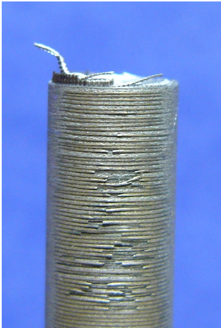
Figure 90 - Sample 13, Configuration 3 after mechanical testing. Exposed W wire was damaged in sample machining before testing.
