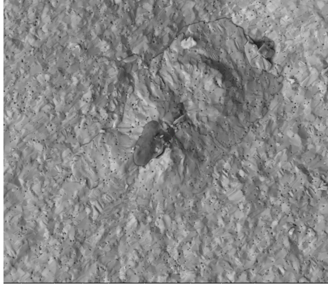
Figure 3.7 Backscattered electron image of a fractured cross-section of \text{La}_{3-x}\text{Te}_4 . The dark area in the center of the image was determined to be Fe/Cr through EDS, which is likely to be contamination from ball milling in the stainless steel vials. The phase impurity and enhanced cracking suggest that this impurity may be the strength-limiting flaw.
