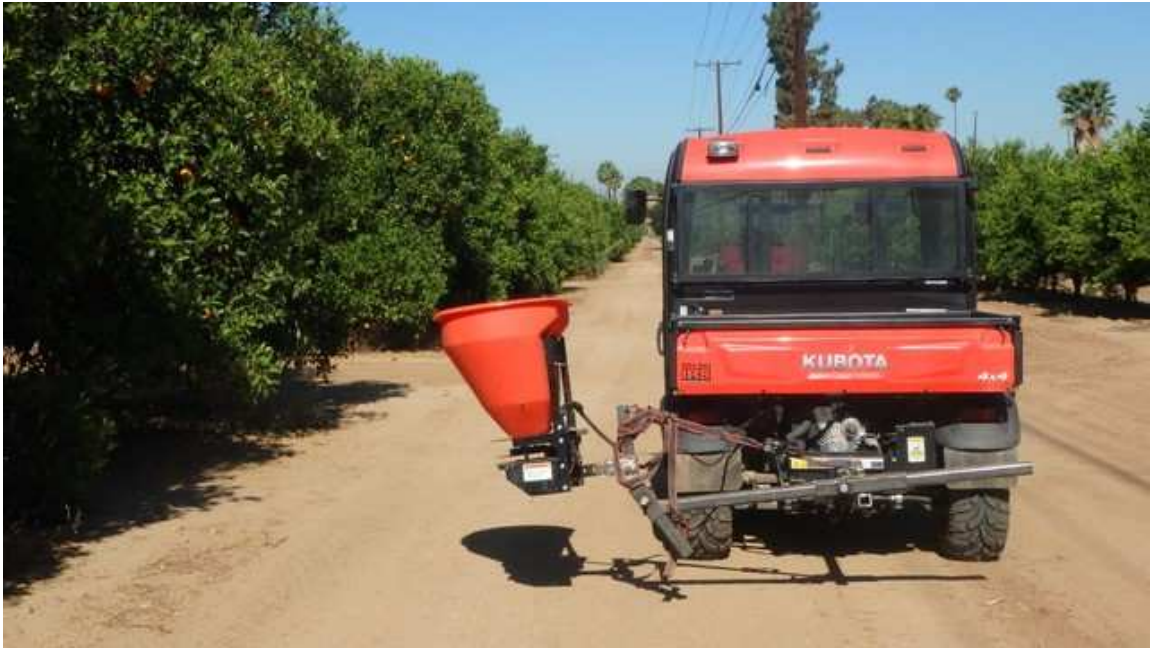
Fig. 4. A utility vehicle with a spreader attached for bait application at the field site.
