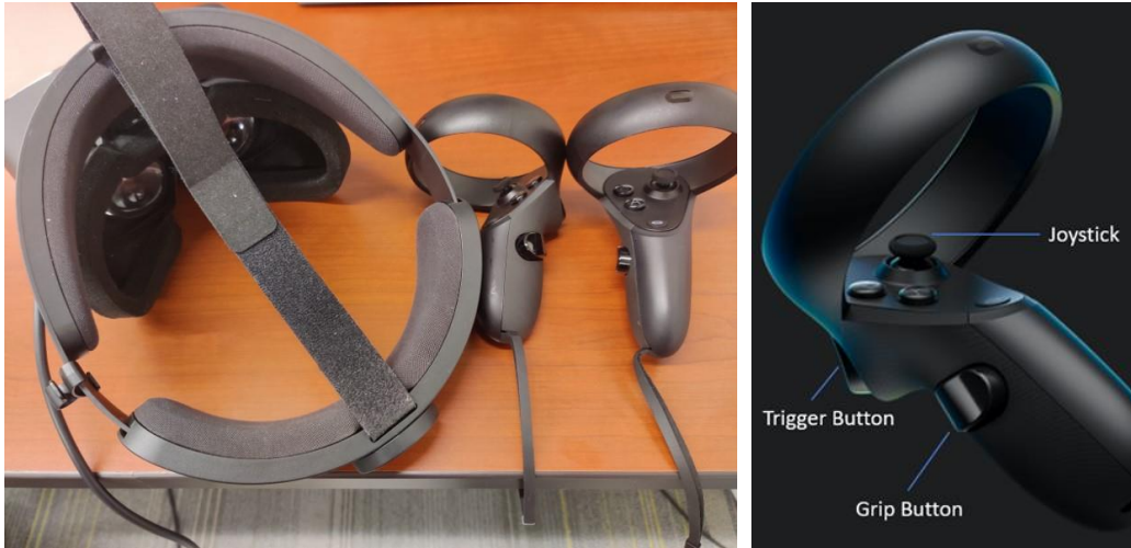
Figure 35. Oculus VR headset and motion controllers with annotations on the three major physical inputs
