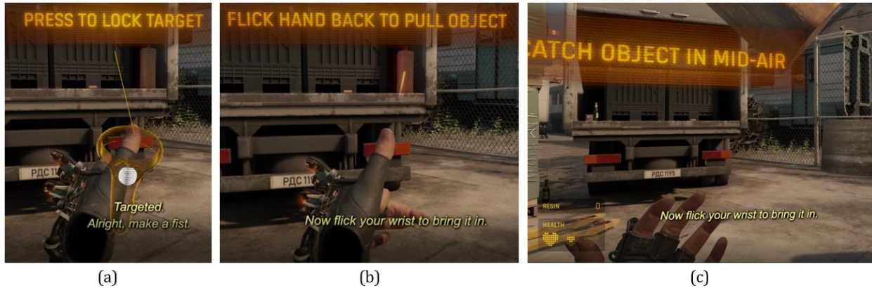
Figure 107. Half-Life: Alyx's hand flicking technique for remote grabbing: (a) point and press trigger to lock target; (b) Once tethered, press the grip and trigger to make a fist and flick hand back to pull object; (c) catch object in mid-air.
