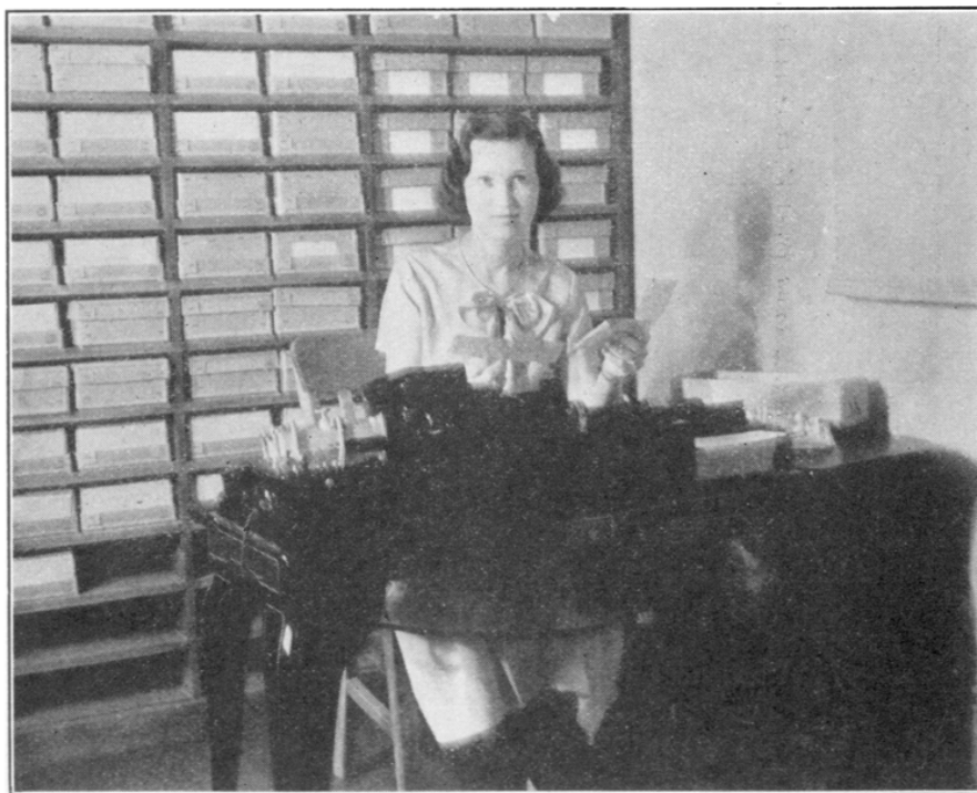
FIG. 8. Electric key punch used in transferring original records to punched cards.
