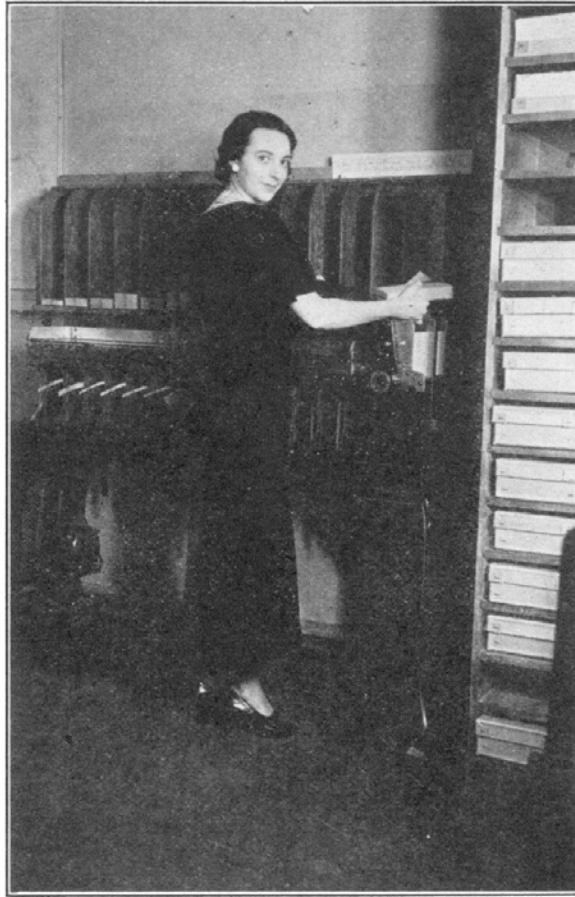
FIG. 9. Electric horizontal sorting machine used to arrange punched cards in proper groupings for tabulating the final reports are referred to the research staff or the law-enforcement officers for investigation. Thus, considerable error is eliminated and organization members are kept in touch with current changes in fishing activities.
