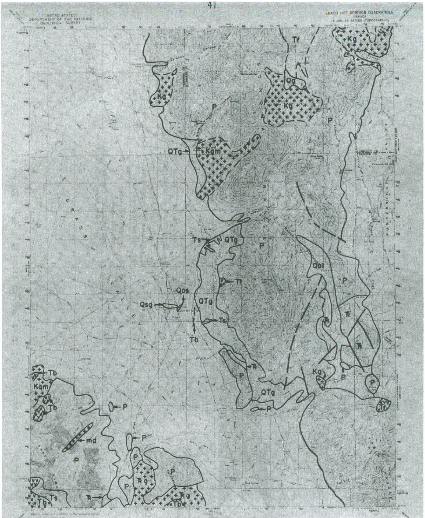
CBB 751-49 Figure 2: Lithologic map, Leach Hot Springs area. Qal: alluvium, Qos: older sinter deposits, Qsg: sinter gravels, QTg: Quaternary-Tertiary gravels and fanglomerates, Tb: Tertiary basalt, Tr: Tertiary rhyolite, Tt: tuff, Ts: Tertiary sedimentary rocks, Kqm: quartz monzonite, Kg: granitic rock, md: mafic dike, TRg: Triassic granitic rocks, TR: undifferentiated Triassic sedimentary rocks, P: undifferentiated Paleozoic sedimentary rocks.
