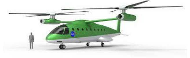
Fig. 2: Six-passenger side-by-side air taxi VTOL concept design from NASA (Ref. 5)
