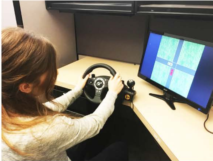
Figure 2.3: Driving Simulator. Top-down view driving simulator with steering wheel and braking pedal.
