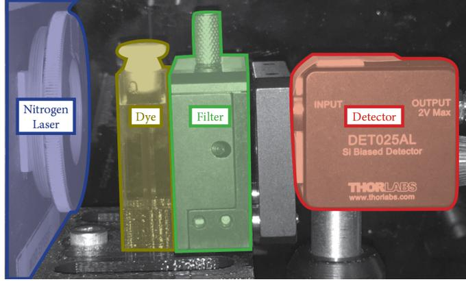
Figure 5.1: Time-domain FLIM dye calibration system setup that consists of the nitrogen laser, dye sample, optical filter, and photodetector.
