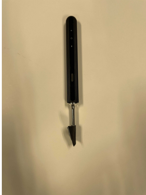
Figure 3.2: Endoscope Camera used for data acquisition with opaque tape modification (Brand: Suear).
