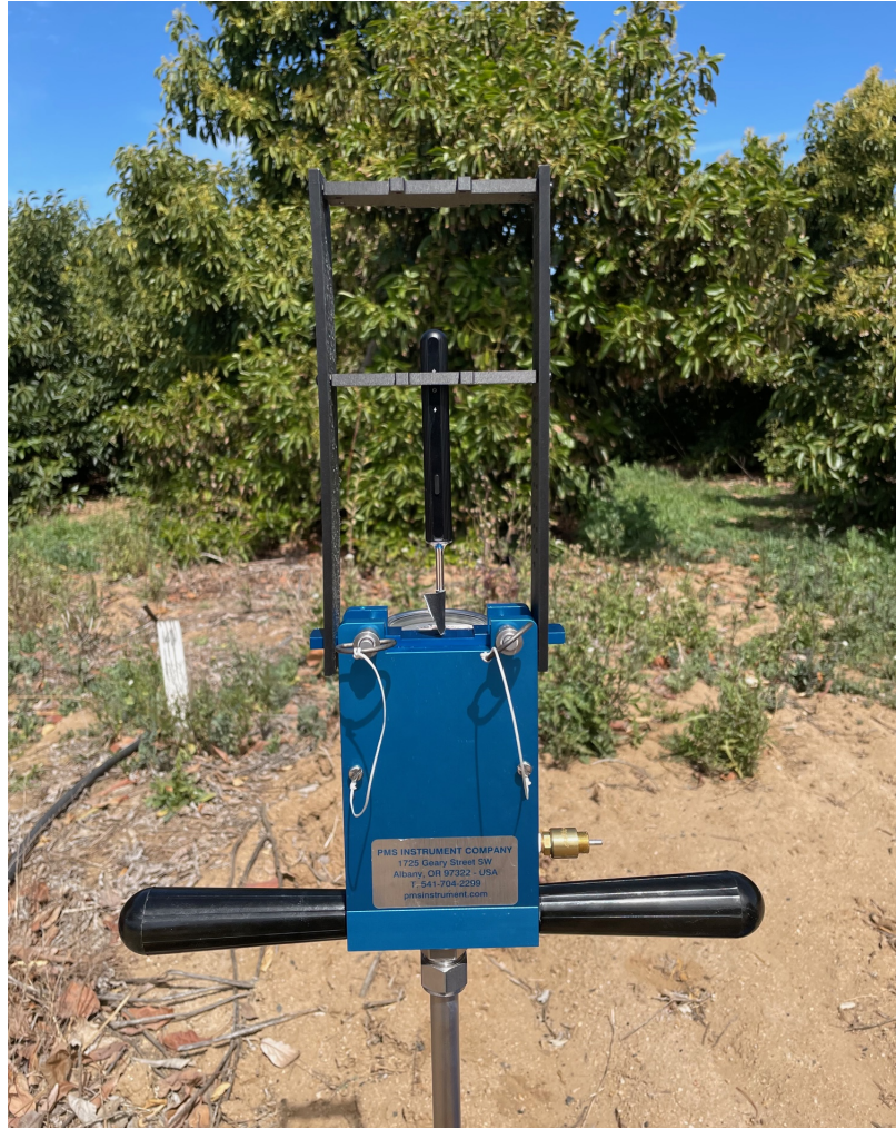
Figure 4.1: PMS pump-up pressure chamber retrofitted with the 3D printed endocam setup, enabling real-time video feed of the xylem during SWP measurements.
