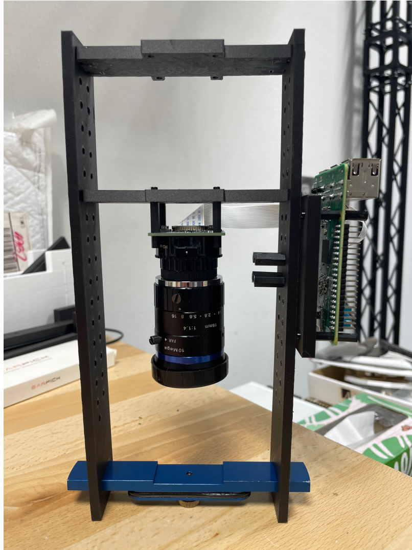
Figure 3.7: HQ Picamera offset lens configuration.
