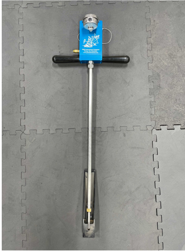
Figure 3.1: PMS Instruments Pump-Up Pressure Chamber (Brand: PMS Instruments).
