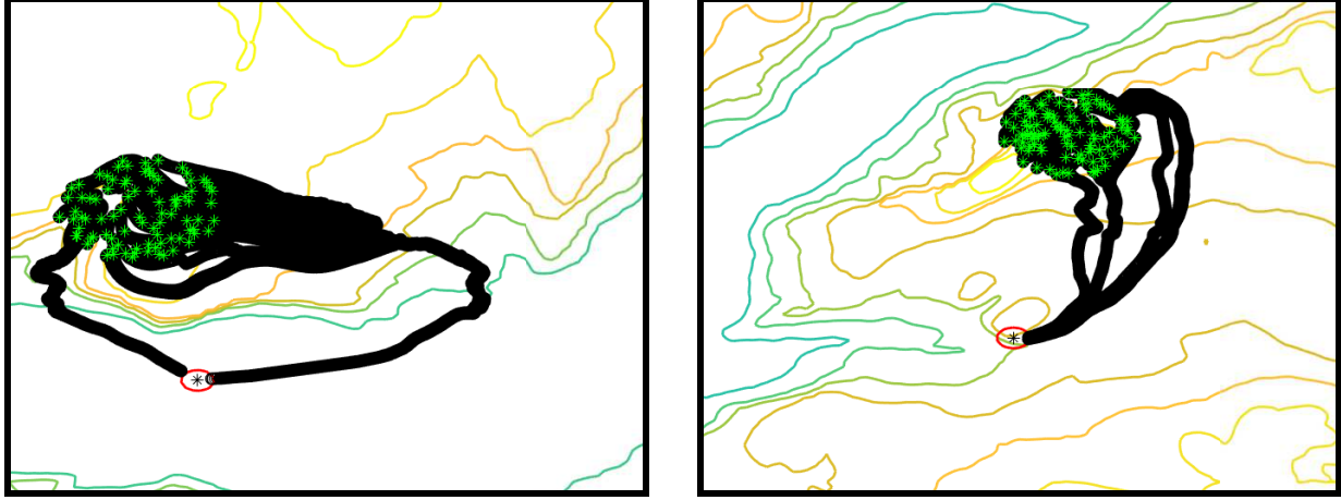
(a) 100 optimal paths traveling down from the summit of El Capitan. (b) 100 optimal paths traveling down from the summit of Half Dome.
