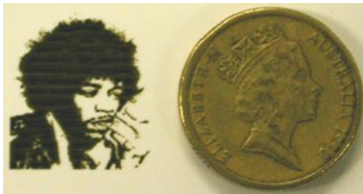
Figure 5.4 A Dimatix printer (top) was used to print an image of Jimi Hendrix (bottom) using a carbon nanotube polyaniline composite ink. Reproduced with permission from ref. 5. Copyright 2007 Royal Society of Chemistry.
