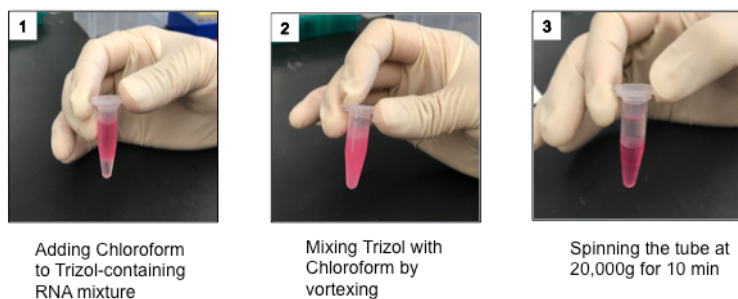
Figure 3: Photographs of mixing phenol-guanidine isothiocyanate reagent and chloroform before and after centrifugation. The mixture is shown when the phenol-guanidine isothiocyanate reagent and chloroform are initially combined, after mixing and after centrifugation. After the mixture is centrifuged, the bottom phase, which is red, is the organic phase. The interphase in the middle is white and cloudy. The top phase is the aqueous phase and it is clear. The RNA is in the aqueous phase, which should be collected with a pipette for precipitation. Please click here to view a larger version of this figure.
