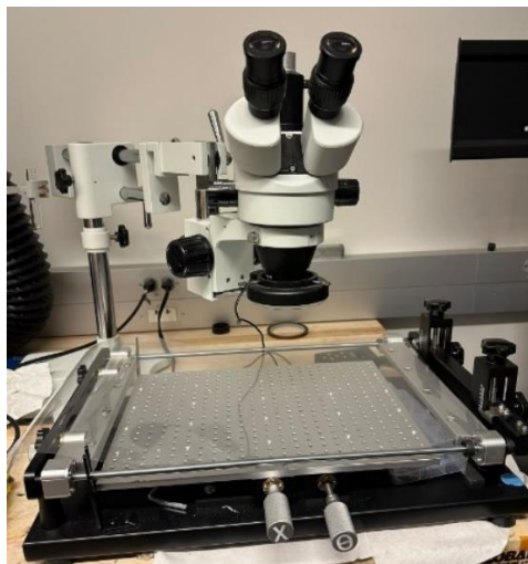
Figure 2-4 NeoDen screen printer used for screen printing electrodes.
