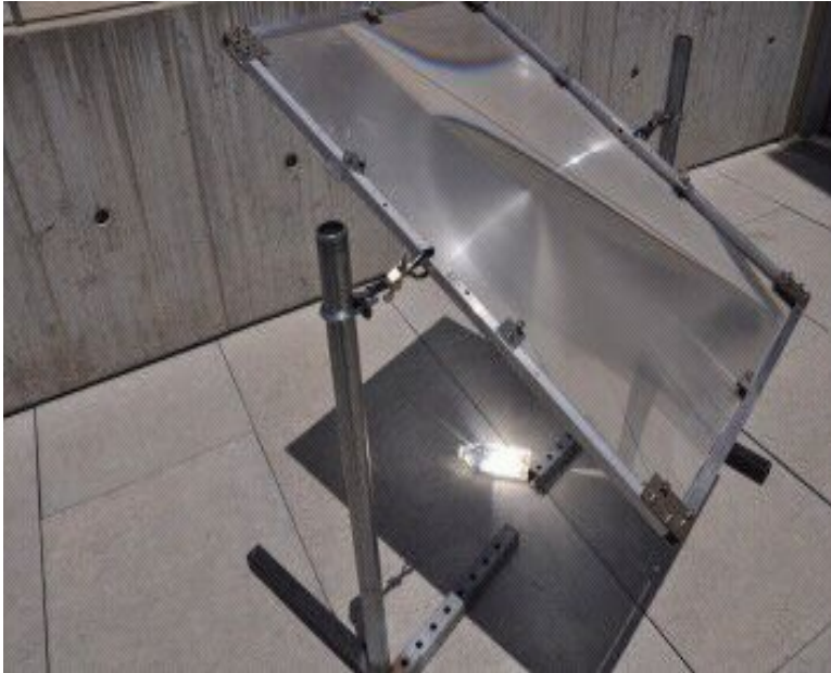
Figure 11: Set up of PULSE method on Dean's patio
