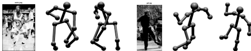
Fig. 2.2 Two 3D reconstructions obtained by Taylor [387], for single orthographic views of human figures. The image appears left, with joint vertices on the body identified by hand (the user also identifies which vertex on each segment is closer to the camera). Center shows a rendered reconstruction in the viewing camera, and right shows a rendering from a different view direction. Figure from “Reconstruction of articulated objects from point correspondences in a single uncalibrated image”, Taylor, Proc. Computer Vision and Pattern Recognition, 2000, © 2000 IEEE.
