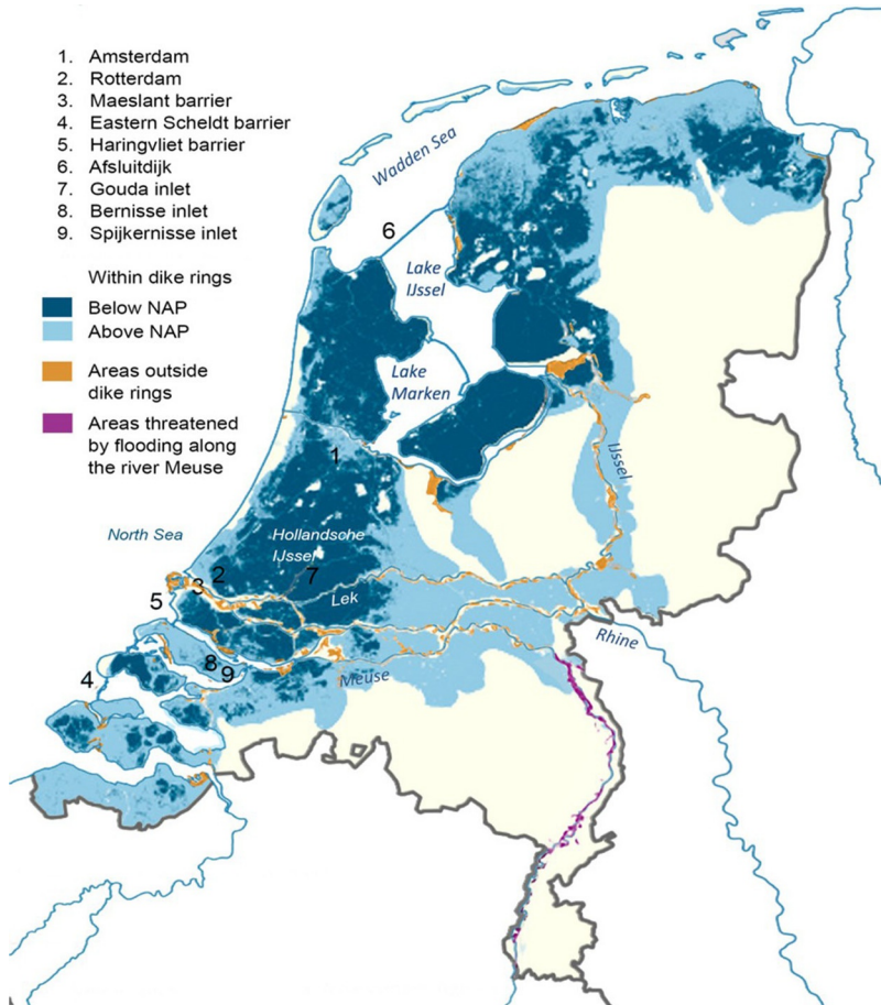
Fig. 31 Current map of the Netherlands. The nine numbers denote locations of the two largest cities, four seawater barriers, and three inlets of fresh river water. NAP stands for sea-level. Protection from flooding by seawater along the coasts is by either dunes or dikes. Used with permission from: PBL Netherlands Environmental Assessment Agency/Rijkswaterstaat-Waterdienst (2010), http://www.pbl.nl .
