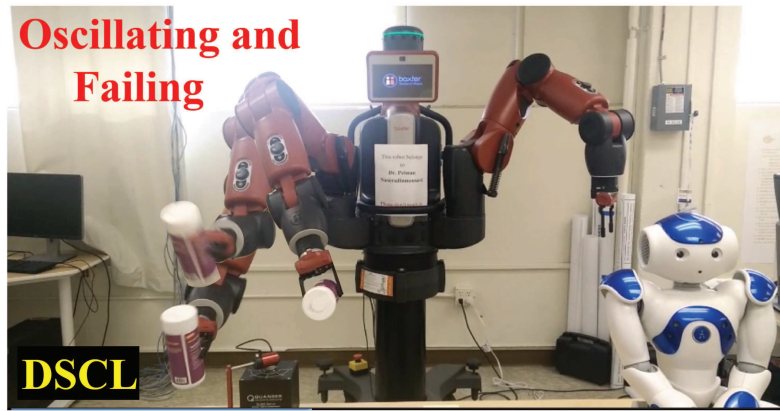
Figure 3.1: The robot fails to track the desired trajectory without a predictor in the presence of input delay
