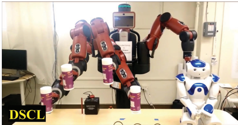
Figure 3.2: A stable obstacle-avoidance pick-and-place task with input delay using the predictor-based controller
