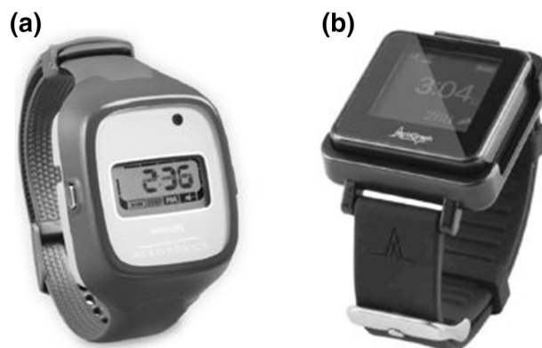
Fig. 2 Examples of wearable medical-grade actigraphy devices, including a Actiwatch Spectrum watch [70], and b the ActiGraph Link GT9X [71]
