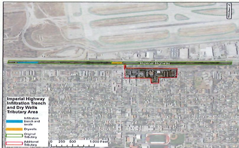
Figure 10. Imperial Highway Sunken Median Stormwater SCM Tributary Area. The project area is the long and narrow rectangular area in the middle of the Figure (green colored).
