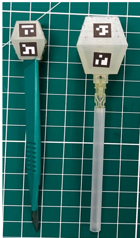
Figure 6.4: Marker attached to surgical instruments
