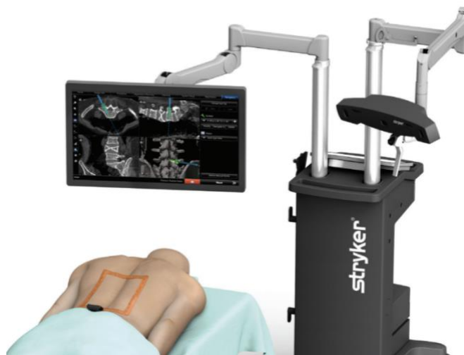
Figure 1.4: Stryker’s surgical navigation solution showing the SpineMask non-invasive tracker on the back and the SpineMap 3D navigation software [14]
