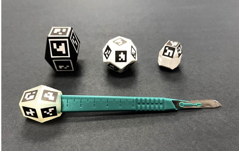
Figure 2.3: 3D ArUco Markers for continuous detection of instruments
