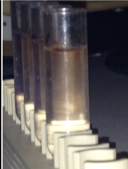
Figure 2.2. Images of CsCl-ethidium bromide DNA binding. The BAC clone DNA was separated into four balanced Beckman centrifuge tubes and centrifuged at 85,000 rpm for 16 hours in a TI-100 centrifuge. The DNA was contained in three small bands and RNA was collected at the bottom of test tube. A, image of DNA bands under UV-light after centrifugation. B, photo of DNA bands after centrifugation taken with a flash.
