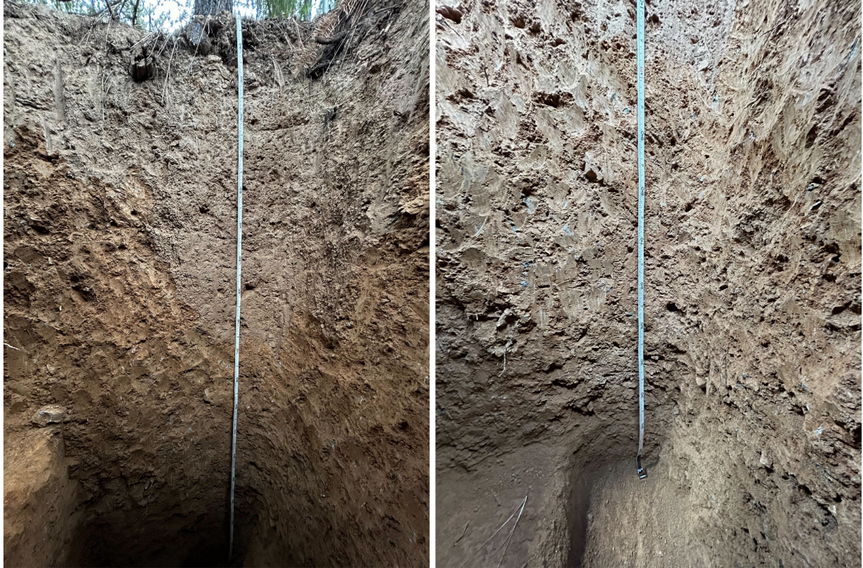
Figure 15. Images displaying upper (left) and lower (right) sections of the 2.0-meter-deep T5 hangingwall excavation with measuring tape for scale (cm).
