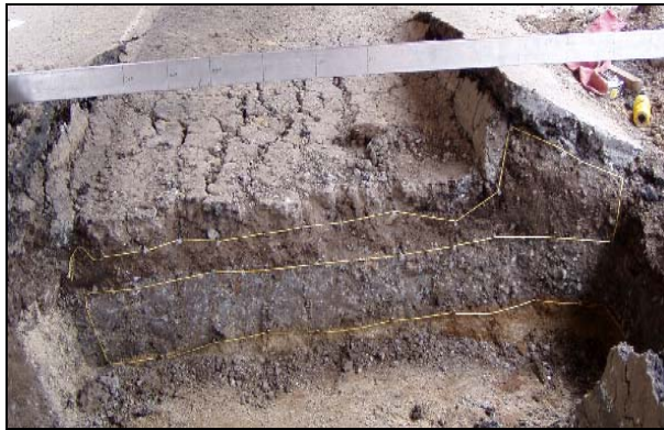
Figure 4.35: Test pit on the completed Section 596FD.
