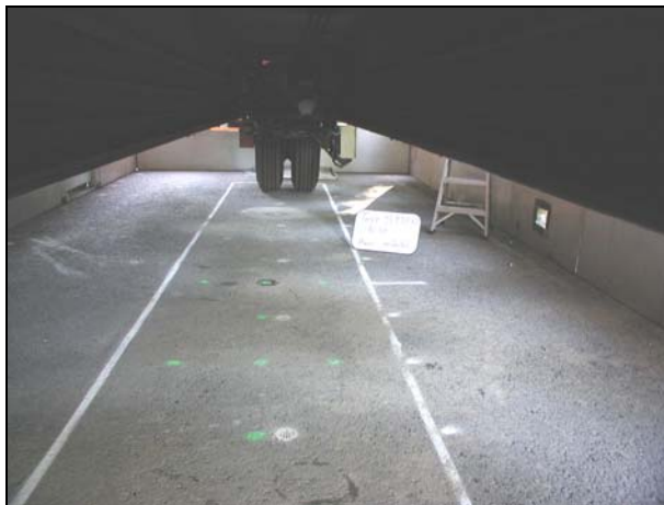
(a) Start of test after 10 repetitions at 60 kN
