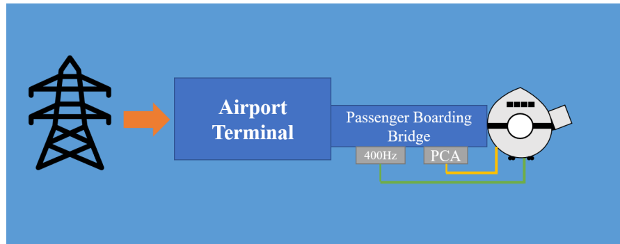
Figure B1: Schematic of 400Hz and electric PCA configuration for parked aircraft.
