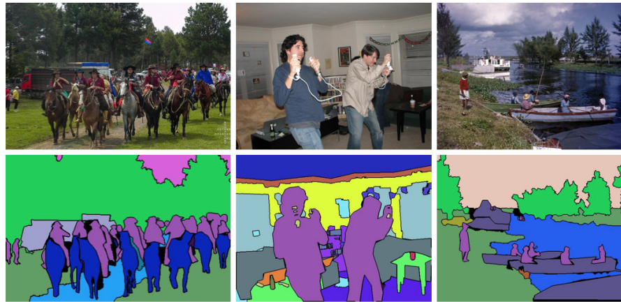
Figure 2.7: Example images and their associated semantic segmentation labels from the COCO Dataset. Each color corresponds to a given class [7].
