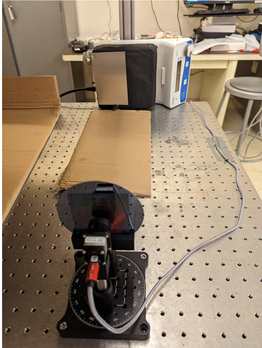
Figure 3.6: Picture of experimental setup. Camera and optic rotate together on stage for MTF measurements, to simulate window being a part of lens optical stack.
