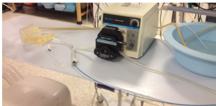
Figure 5. Closed flow loop setup for acquiring DSA images of the patient-specific vascular flow phantom.
