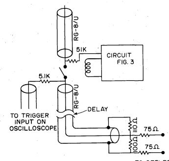
IOOΩ & IIOΩ RESISTORS ARE SYMMETRICALLY CONNECTED WITH MINIMUM LEAD LENGTH. 75Ω RESISTORS CONNECT FROM CABLE TO TUBE CLIPS WITH MINIMUM LEAD LENGTH. TO DEFLECTION PLATES OF TYPE 5XP CATHODE RAY TUBE
