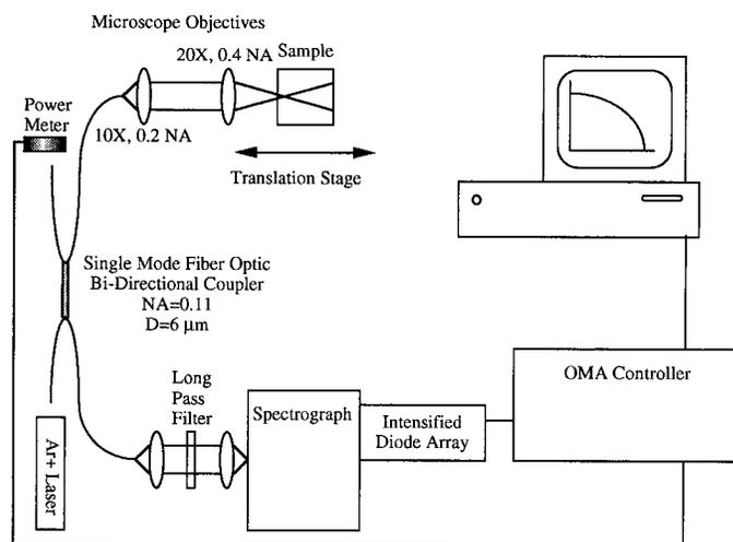
FIG. 1. Block diagram of the fiber-optic confocal spectrometer.
