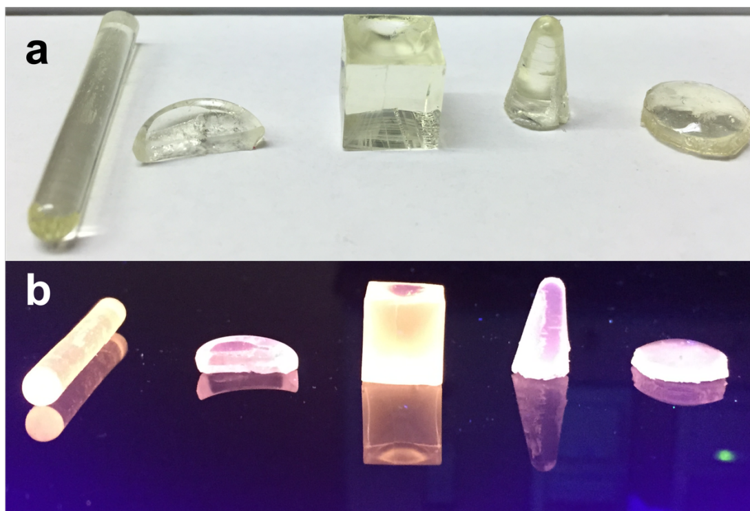
Figure 2.II.14. (a) Images of the photoactivated CO-releasing polymer under visible light and (b) under UV light (365 nm). The polymer is composed of complex 1 covalently attached within polymeric matrix of pHEMA/EGDMA. The intense luminescence of 1 can be detected qualitatively indicating the amount of photoCORM remaining within the polymer.
