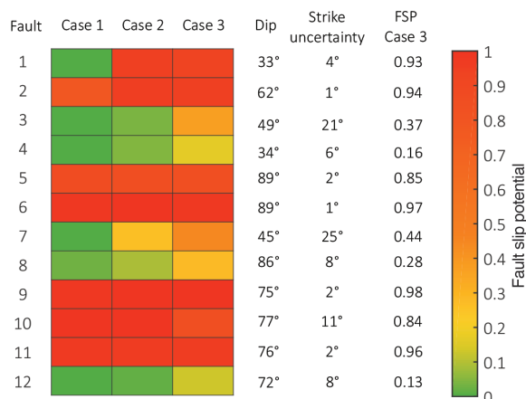
Figure 8. FSP after Walsh and Zoback (2016) for faults derived from hypocenter locations for different assumptions of the accuracy of the resolved strike and dip. Case 1 assumes strike and dip as resolved from earthquake hypocenters. Case 2 assumes dip of 85^\circ \pm 5^\circ and strike as resolved from earthquake hypocenters. Case 3 assumes dip of 85^\circ \pm 5^\circ and strike and its 2\sigma -error.
