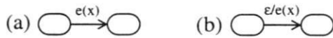
Figure 7. (a) A CSP event with input data, e?x , is modeled in UML State Machines as a state transition event with no action. (b) A CSP event, e , with output data, e!x , is modeled as a null state transition event that results in action e .
