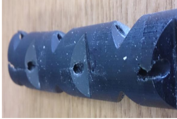
Figure 57: Melt points in the endoscope design (point arrow to tear point)
