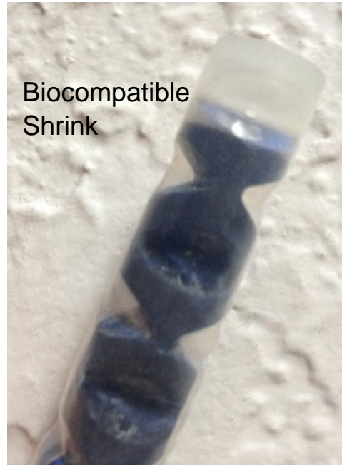
Figure 36: The v-groove endoscope assembled with a biocompatible shrink
