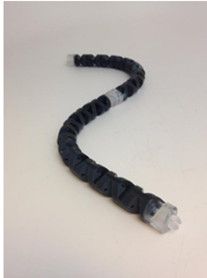
Figure 34: 3-D printed follower for v-cut groove design
