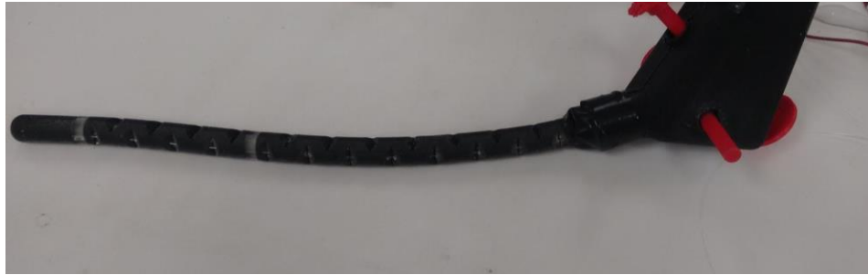
Figure 35: 3-D printed design for v-cut groove endoscope
