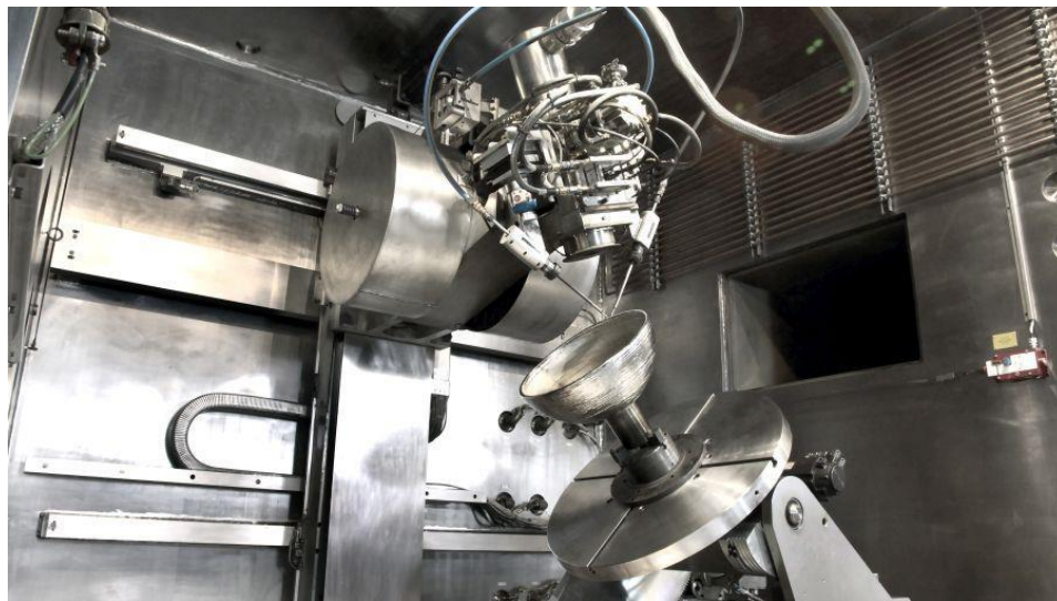
Figure 10: EBF 3-D printing of steel [16]
